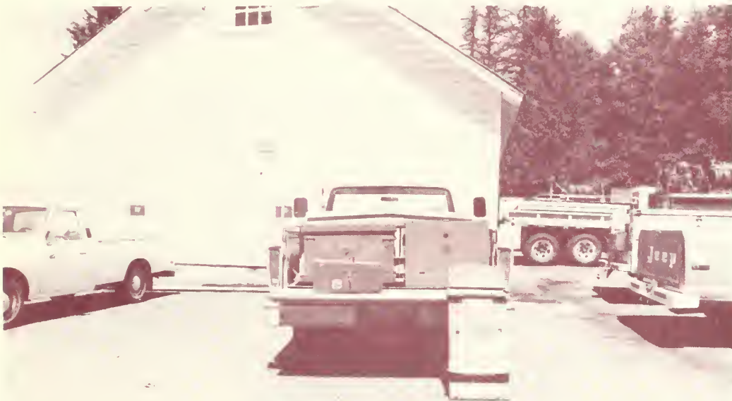
Figure 2. Field-going microwave outfit ready for transport. Oven is on the left, generator on the right. Small box contains scale. Shock mounted platform would be in place under oven during transport.
