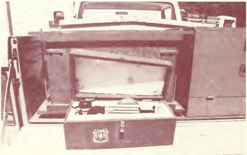
Figure 3. Thick foam rubber cushions the oven during transport.
