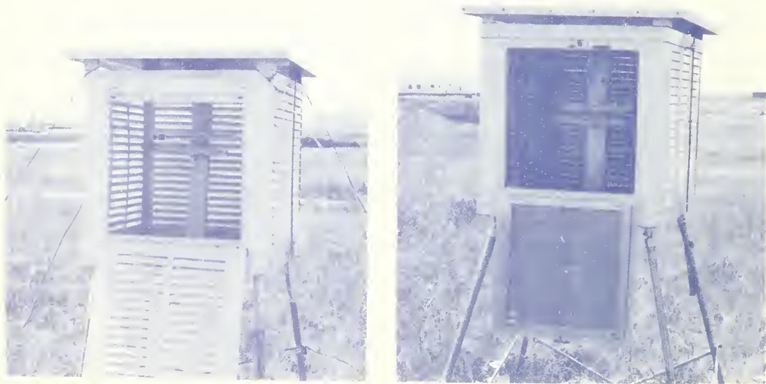
A1 Figure 1.--Closeup of new model aluminum shelter, A2, and older aluminum shelter, A1, showing difference in louver construction and the unpainted interior of A2.
