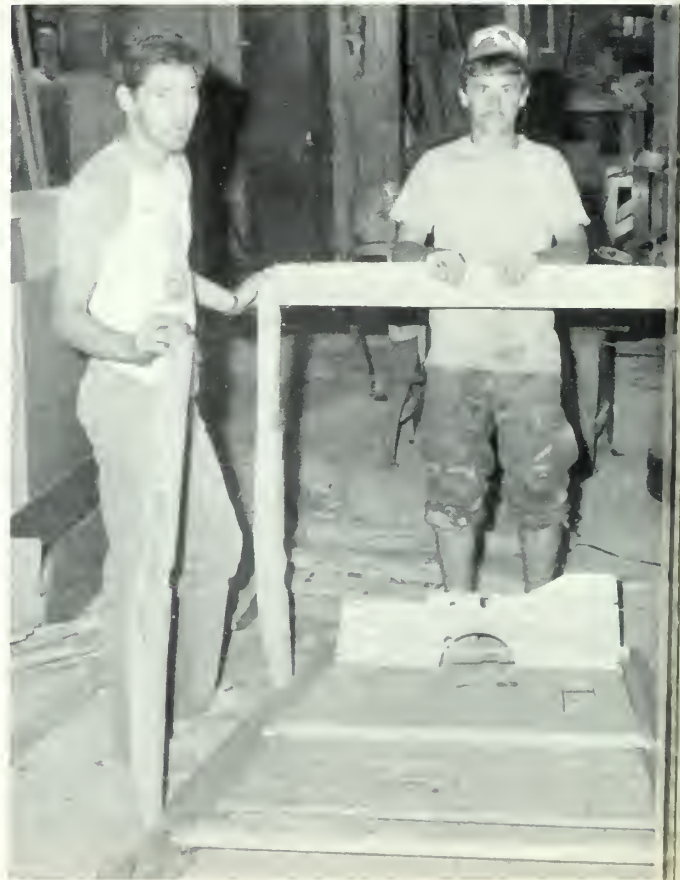
Wood technicians Tim Crumbley (left) and Kenneth Matheson (right) assemble wooden car frame. The technicians are employed by the South Georgia company that specializes in wooden car parts. A wooden auto frame shown is subflooring custom-built 1932 model Chevrolet
