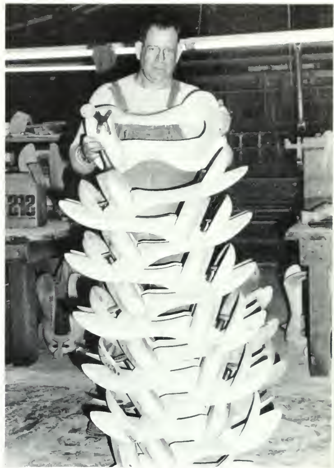
At left, manager of Flor Saddle Tree Company, checks dimensions of Southern yellow pine saddle tree with customer. Established in 1879, the company is the only one of its kind in the state and possibly oldest such organization in the nation. At right, veteran saddle tree craftsman Earl Watson displays stack of wooden saddle trees ready for rawhide stitching and leather covering. Although it is not obvious by looking at the finished product, a saddle made of more than half wood. The requirements of this specialized woodcraft have changed little since the days of the Old West.
