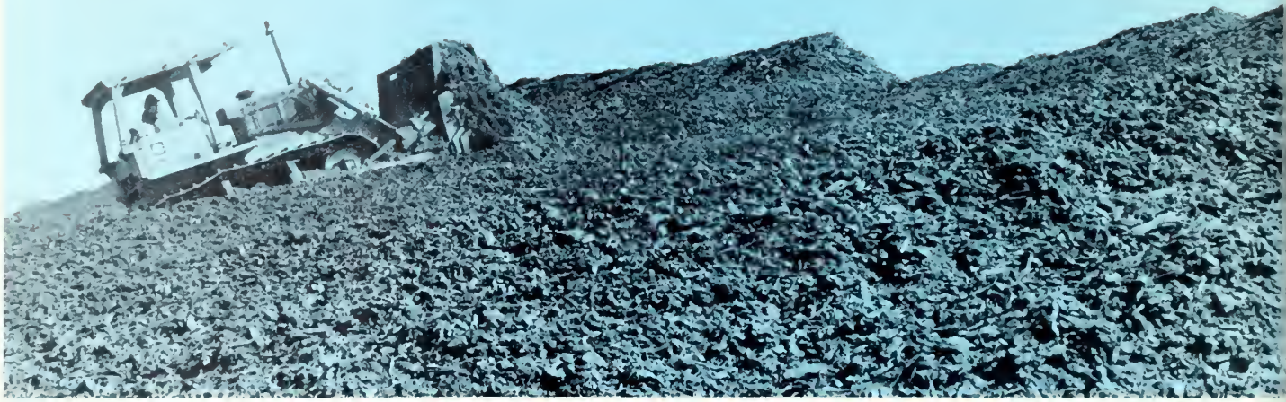
A bulldozer turns tree bark to prevent temperature buildup. Below, an automatic unloader accommodates one of many bark hauling trucks.
