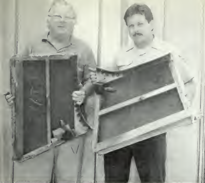
Businessman Jim Tygart (left) and Monroe Gaines, Commission ranger for Berrien County, display wooden frames of car doors that were typical on most autos until 1937.
