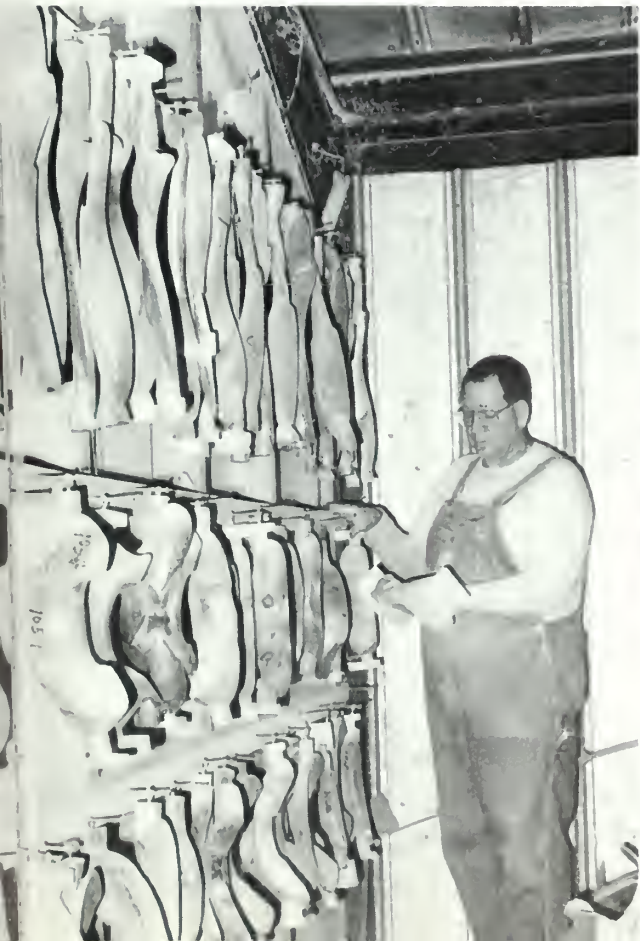
At left, Watson checks oak patterns for saddle trees. More than 600 wooden models are stocked by the Demorest based company. Many of the company's personnel are third and fourth generation craftsmen. Saddle tree craftsman shown above attaches horn to wooden saddle tree. Although automated tools are used, wood craftsmen spend as much time using sandpaper and a hand rasp as they do operating power tools.
