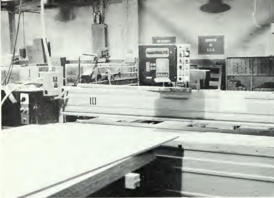
A computerized table saw that stores cutting instructions assures clean and uniform sawing of wood product.
