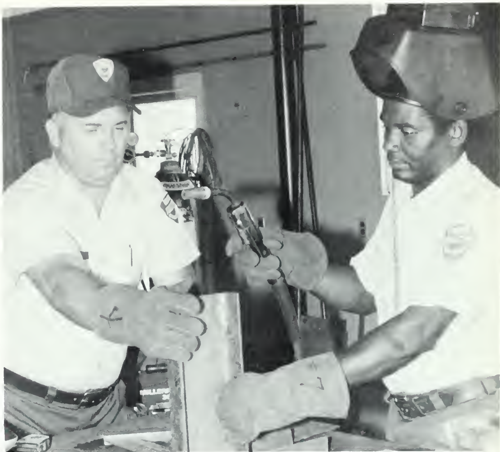
Forest Patrolmen Larry Womack, left, and Sam Williams weld a section of metal to be used in the construction of a fire truck tank. The modern shop at the unit builds tanks for the Rural Fire Defense program, a project that provides equipment for volunteer fire departments mainly in Georgia's rural areas.
