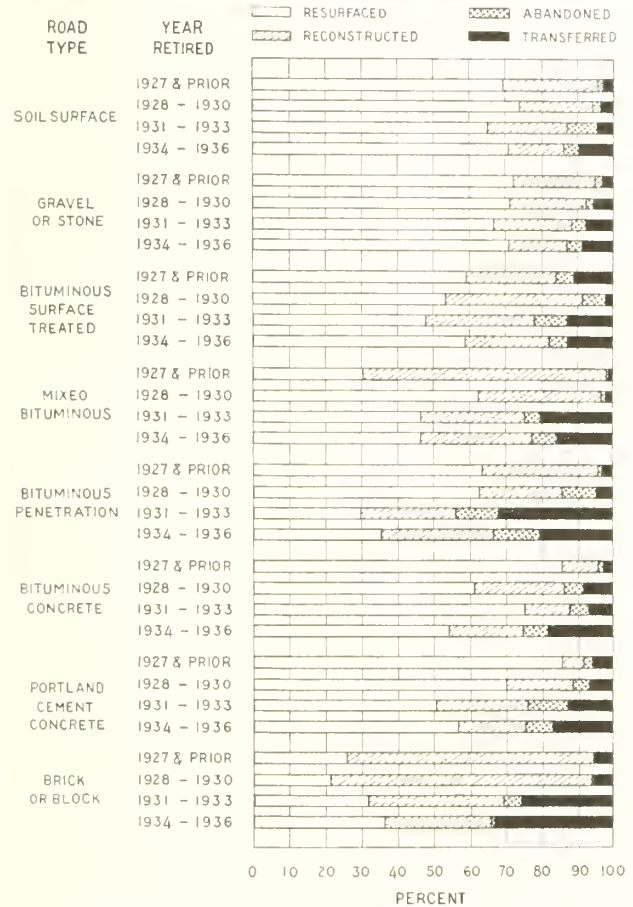
FIGURE 12.—METHODS OF RETIREMENT OF VARIOUS TYPES OF ROAD SURFACES FOR FOUR GROUPS OF YEARS.
