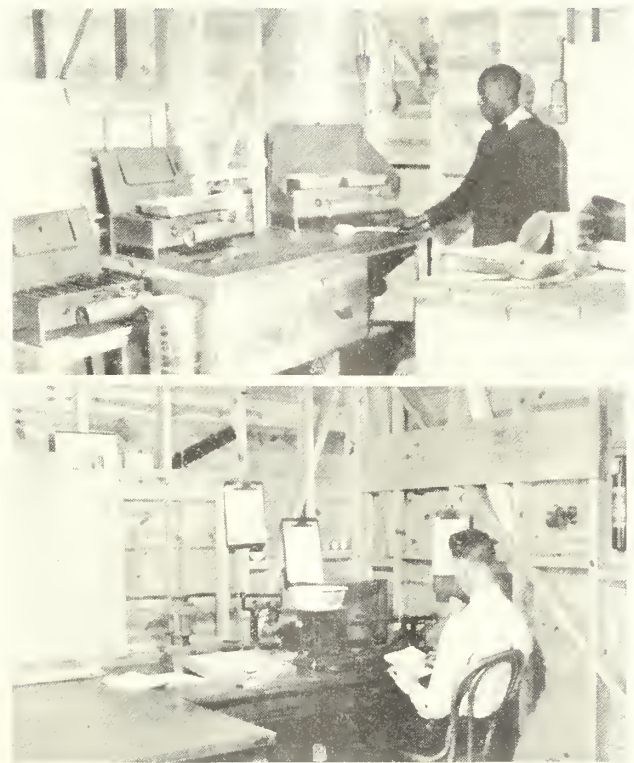
FIGURE 15. LABORATORY TESTS ON SAMPLES. A, DRYING GRAVEL SAMPLES ON DOUBLE-BURNER GASOLINE CAMP STOVES; AND B, DETERMINING WEIGHTS OF MATERIAL RETAINED ON VARIOUS SIEVES.
