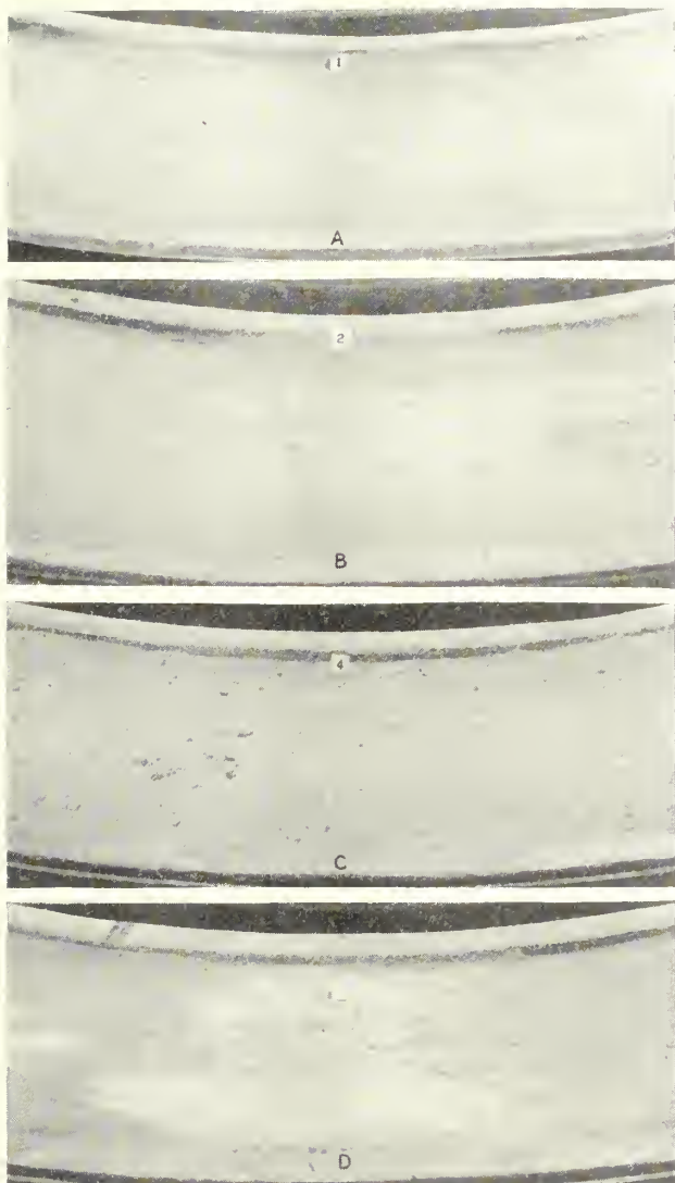
FIGURE 3.—APPEARANCE OF TEST SECTIONS AFTER 202,600 WHEEL-TRIPS OF DISTRIBUTED TRAFFIC ON THE UNTREATED MATERIAL. A, SECTION 1; B, SECTION 2; C, SECTION 4, WHICH IS ALSO REPRESENTATIVE OF THE APPEARANCE OF SECTION 3; AND D, SECTION 6, WHICH IS ALSO REPRESENTATIVE OF THE APPEARANCE OF SECTION 5.
