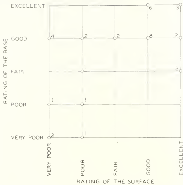
FIGURE 8.—RELATION OF SURFACE CONDITION TO BASE CONDITION. (NUMERALS INDICATE NUMBER OF SECTIONS.)
