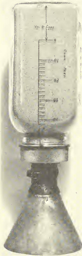
FIGURE 21.—SAND JAR WITH FUNNEL FOR USE IN SOIL DENSITY DETERMINATIONS.
