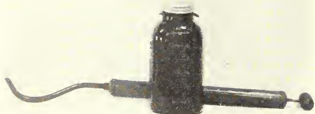
FIGURE 22.—OIL JAR AND PUMP FOR USE IN SOIL DENSITY DETERMINATIONS.
