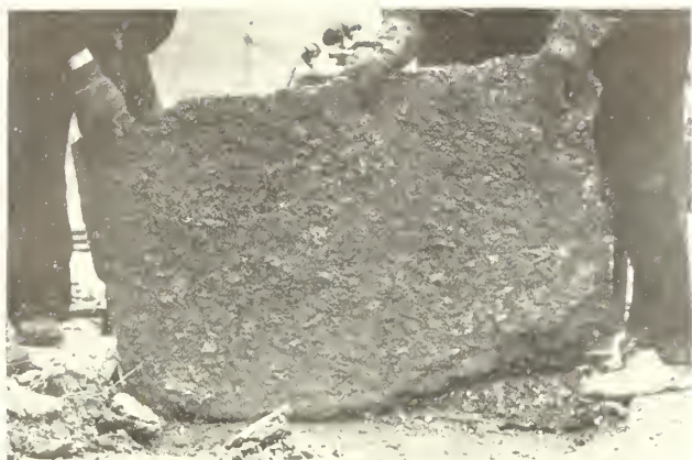
FIGURE 1.—A TYPICAL FIELD SAMPLE OF BITUMINOUS CONCRETE SURFACING.
