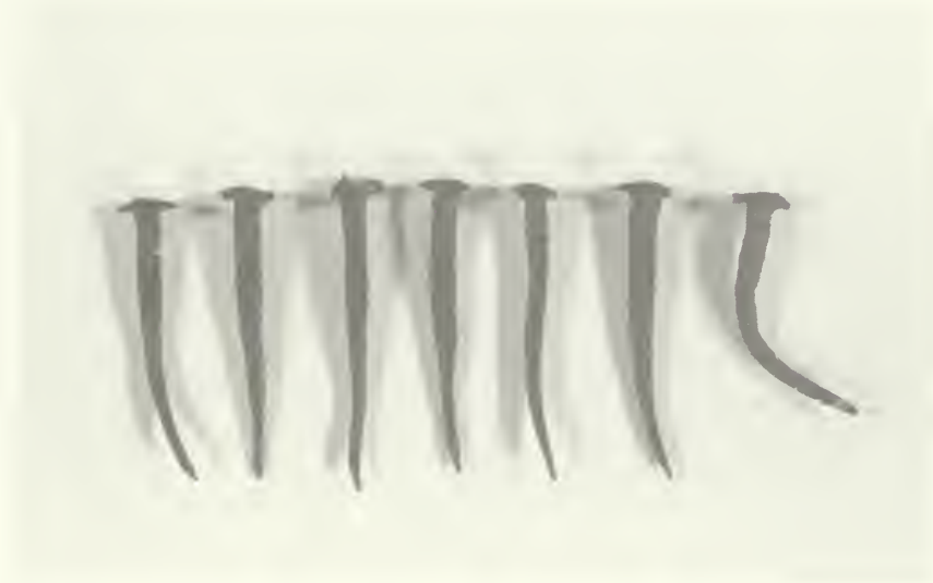
Photograph No. 5: 8d (2-1/2 inch) wrought nails with rose heads, ca. 1730
