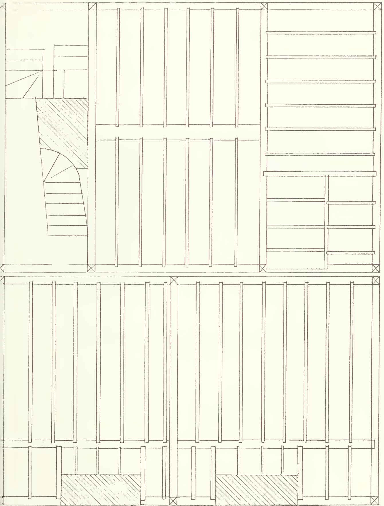
Illustration 21. Antram-Gray House: Second-Floor Framing Plan.
