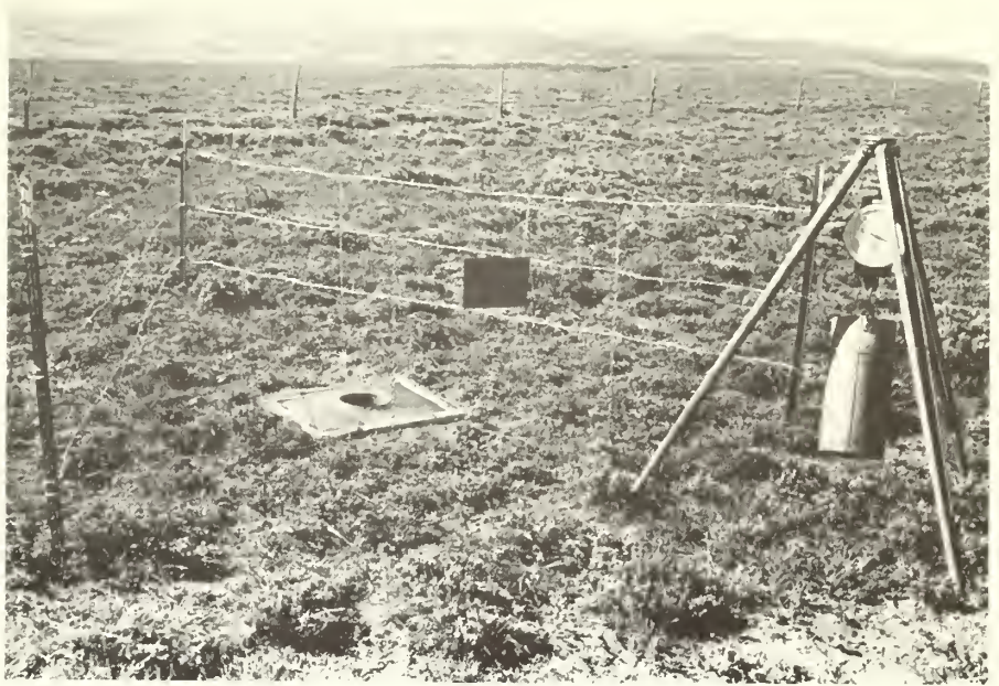
Figure 2.—A functioning sleeved pit gage in a typical windswept situation.
