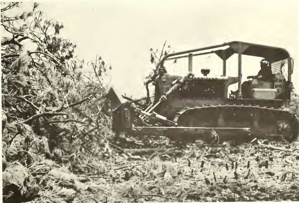
Figure 4.—Tractor with automatic transmission and a hydraulically controlled blade with rake teeth windrowing slash.
