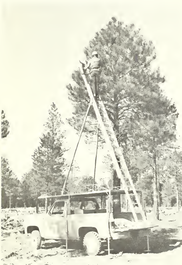
Figure 2.—The base of the extension ladder is attached to brackets on the truck tailgate by steel pins. Note reinforcement of ladder above the point of attachment and wide steps on the ladder.
