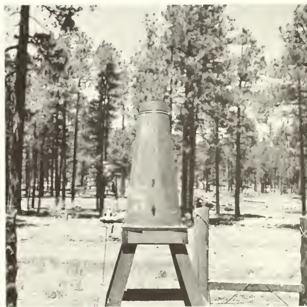
Figure 1.—A 100-inch Sacramento storage gage in use on the Beaver Creek watershed, Arizona.
