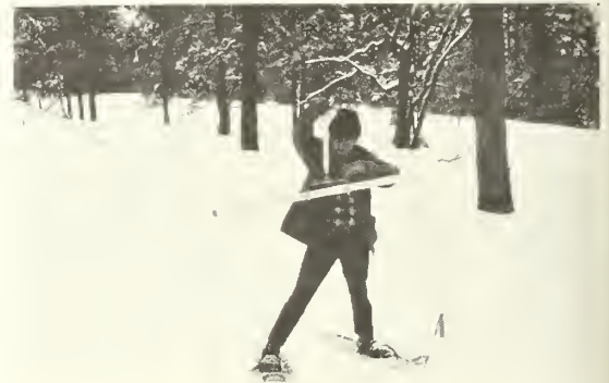
Figure 2.—Determining water equivalent of snowpack with a Federal snow sampler and scale.
