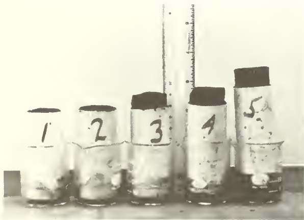
Figure 6.—Soil cylinders at the conclusion of a 10-day freezing experiment. Note that the soil column has heaved out of the bottom of the cylinders also, especially those on the right.
