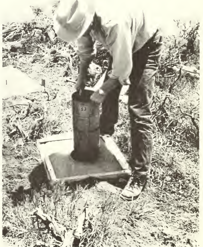
Figure 3.—The gage can be easily lifted out of its sleeve for servicing.
