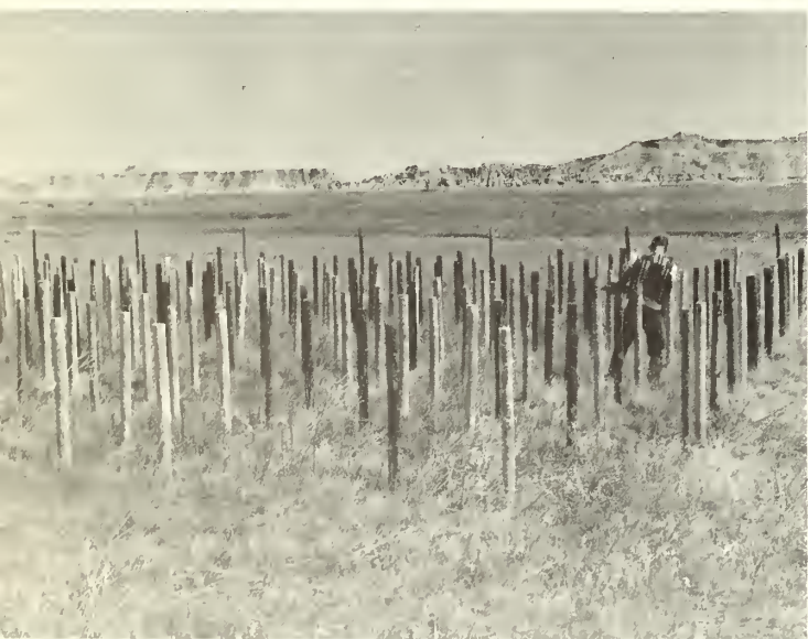
Figure 3.—The well-drained plot near Scenic has a clay soil with a pH of 7.4. This plot has no washed-in soil. Posts are being tested with the 50-lb lateral pull.
