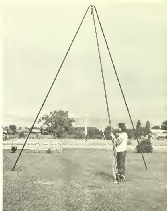
Figure 2.—Tripod mount equipped with 21-foot-long, 1½-inch pipe legs and block and tackle.
