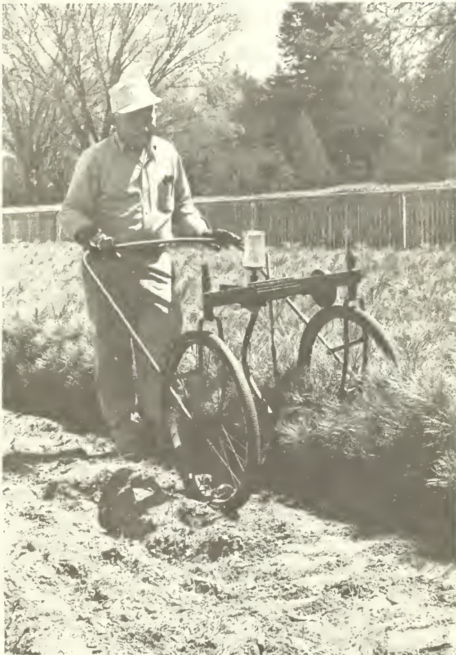
Figure 2.—Insecticide applicator, fabricated from front bicycle forks, two bicycle wheels, and a Nometering device, delivered granules through a garden hose to the soil surface in a 6-inch-wide band.
