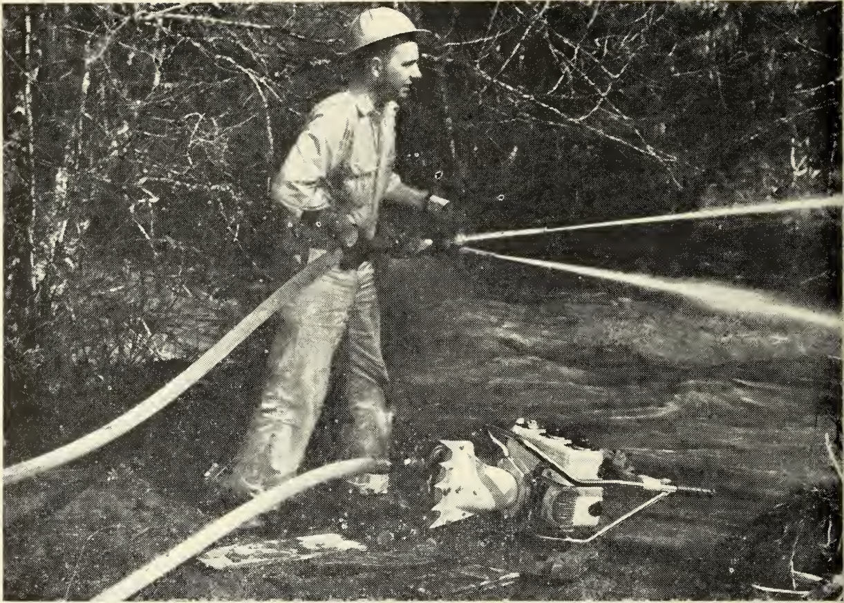
FIGURE 2.—Cecil Cunningham, Weyerhaeuser Timber Company forester, Springfield, Oreg., demonstrates power-saw fire-pump combination. In fighting actual forest fire, two hoses, each fitted with nozzle, would be used.
