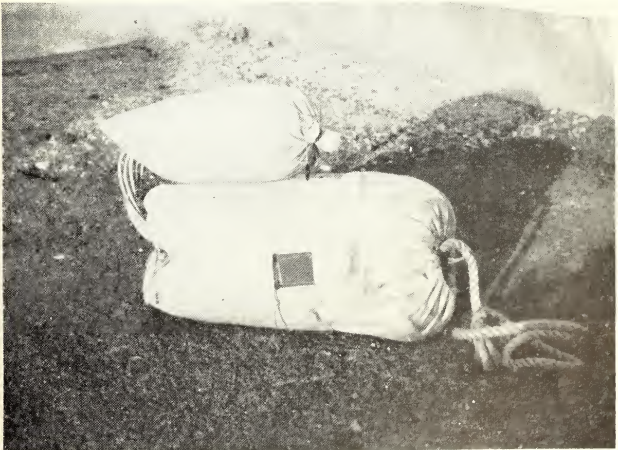
FIGURE 1.—Long-rope parachute with pilot chute.
