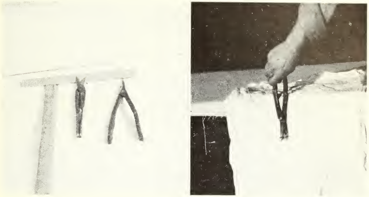
FIGURE 2.—Hog ring spreading tool showing its size and how it operates to spread a hog ring.
