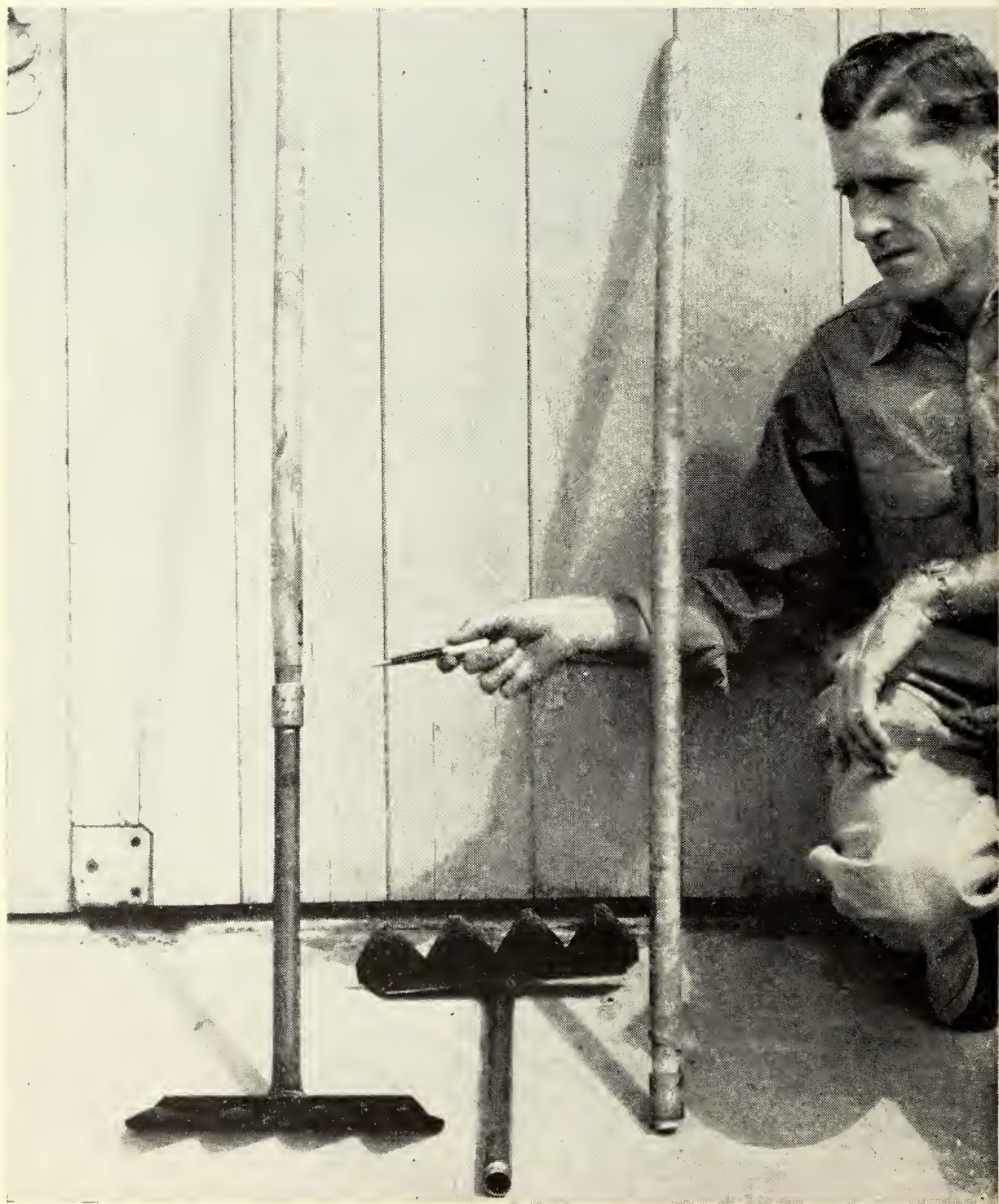
FIGURE 1.—View of Council rake showing the assembled and unassembled knock-down handle. (Photo courtesy Indiana Dept. Conservation.)
