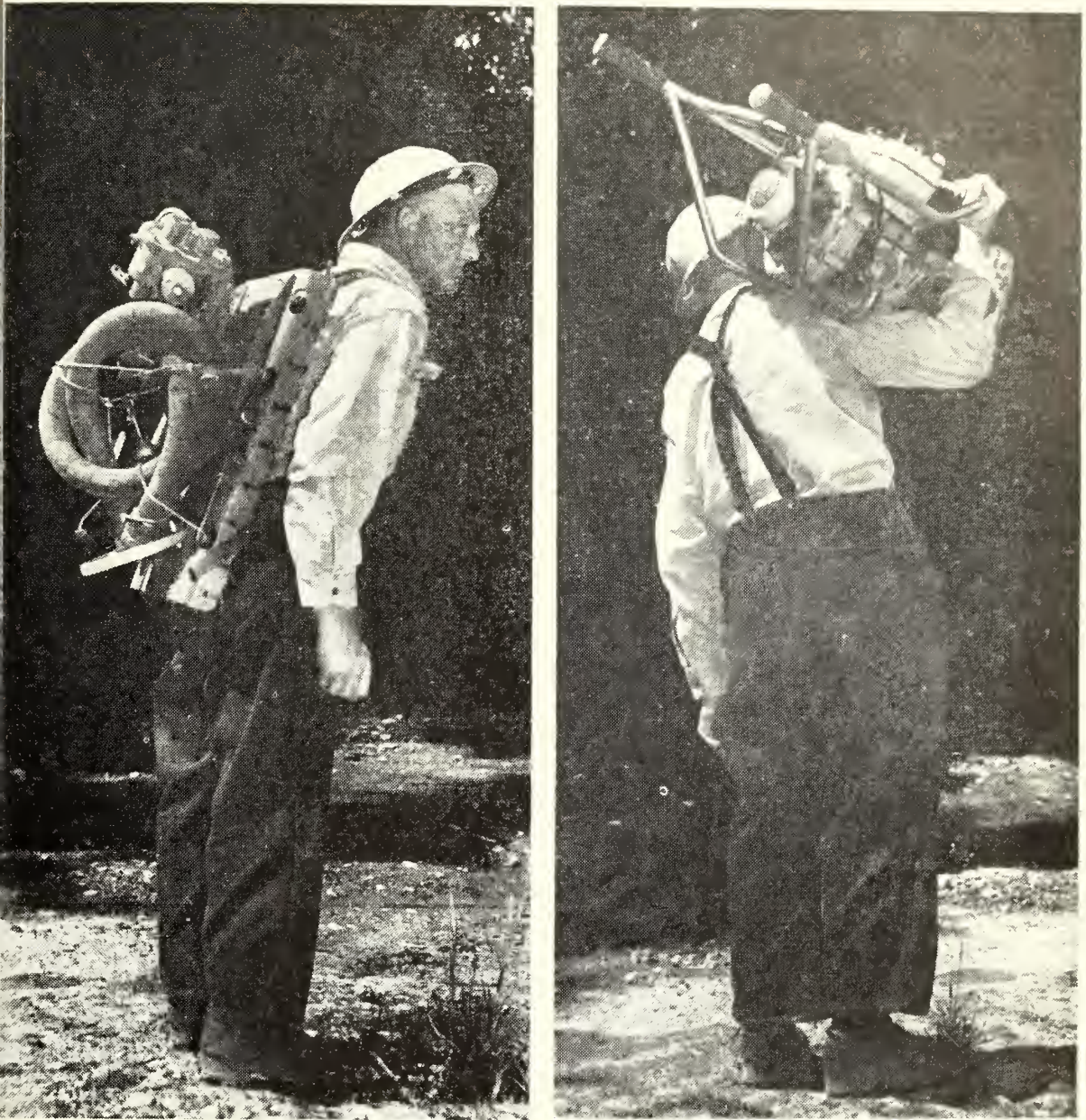
FIGURE 3.—Power-saw fire-pump combination is a two-man load. Robert Gehrman, who invented the coupling by which pump is attached to power-saw motor, demonstrates: Left , carrying pump on a packboard; right , packing power-saw motor.
