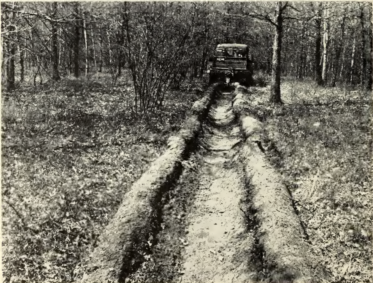
FIGURE 3.—Clean wide line made by power-wagon plow.
