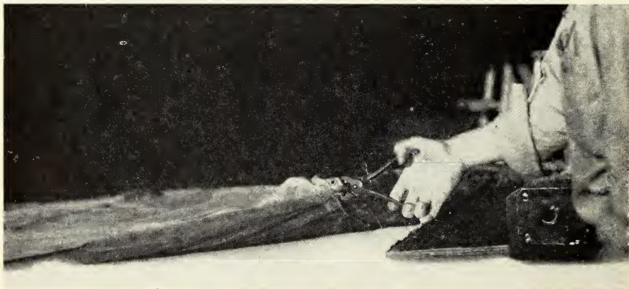
FIGURE 1.—Inserting a hog ring through the eyes placed in the separate parts of a kapok sleeping bag. When in place all parts are fastened securely together with the closed ring.
