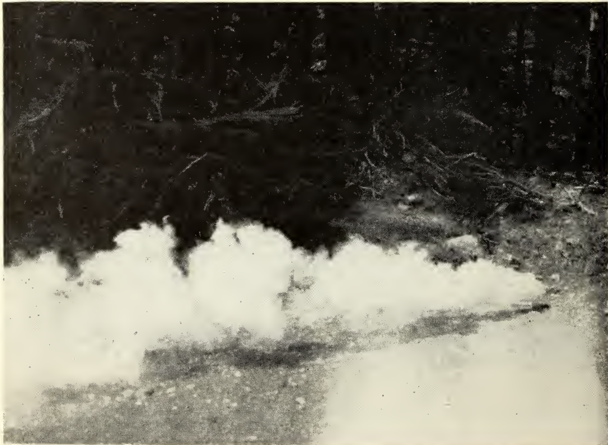
FIGURE 1.—Smoke produced by a candle. There was no noticeable wind in the deep timber, but natural draft along the roadside was sufficient to “pull” the smoke horizontally. In this case the smoke did not rise above the trees.
