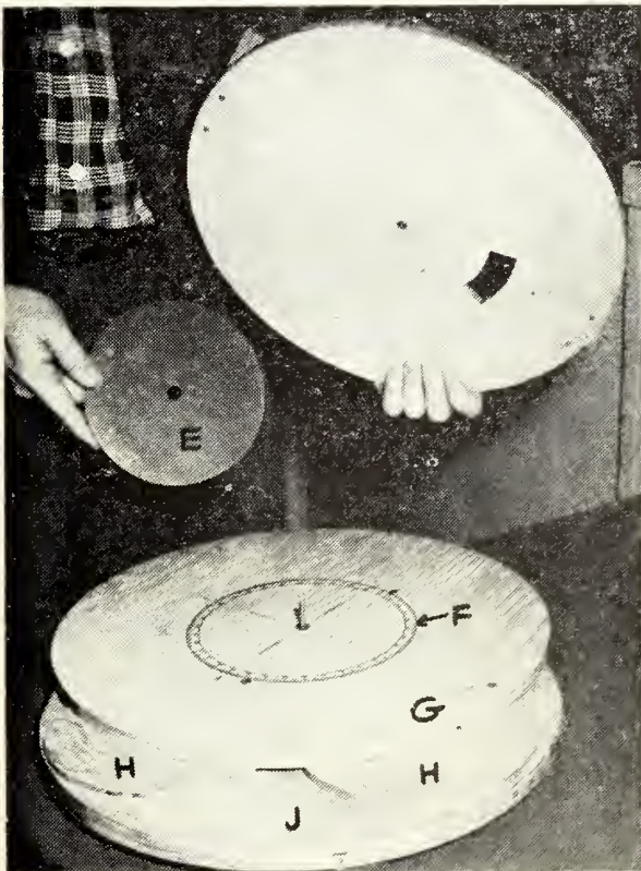
FIGURE 1.—Three views showing component parts of the Kentucky fire finder.
