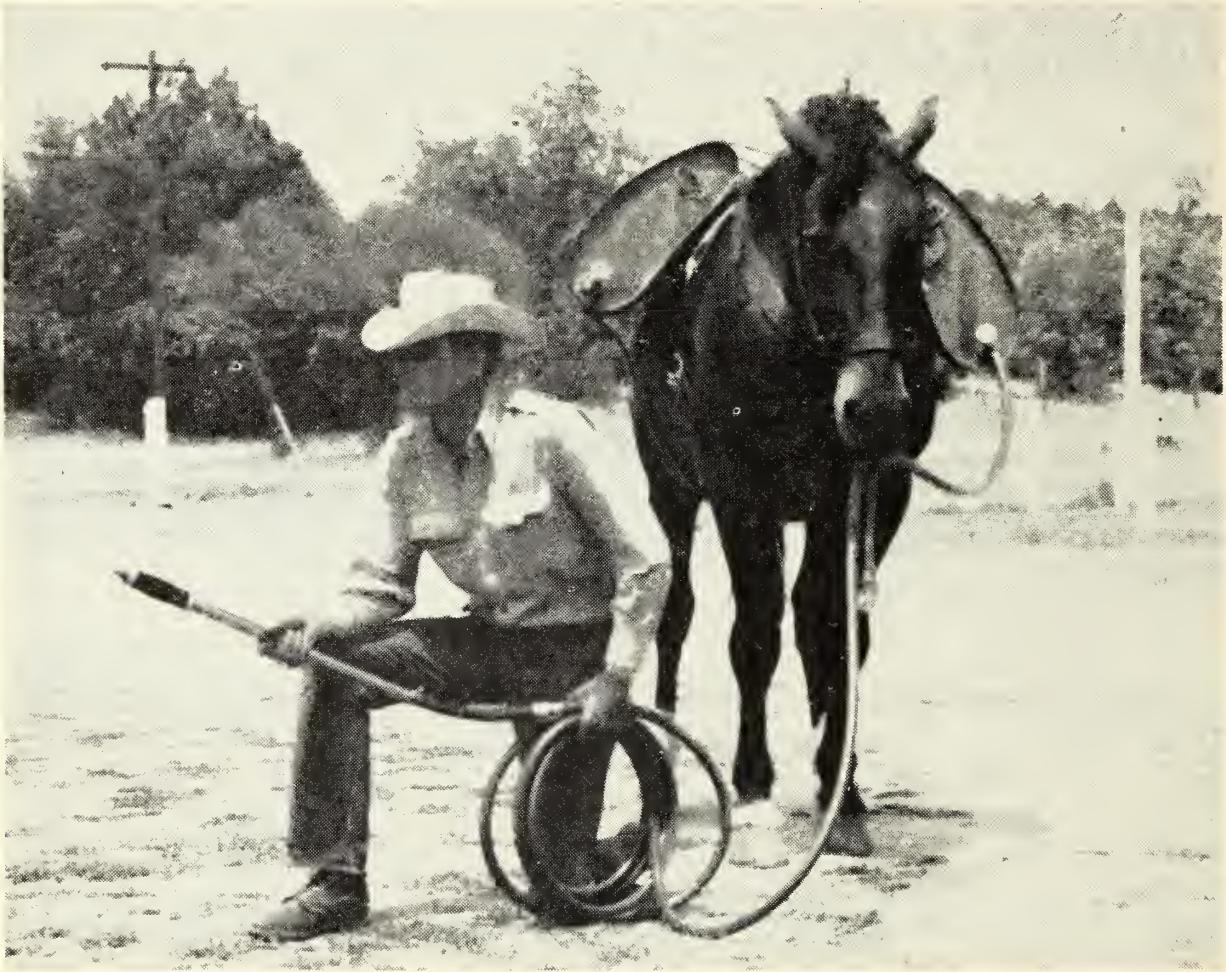
FIGURE 1.—Water pack cans in place with hose and pump ready for use.
