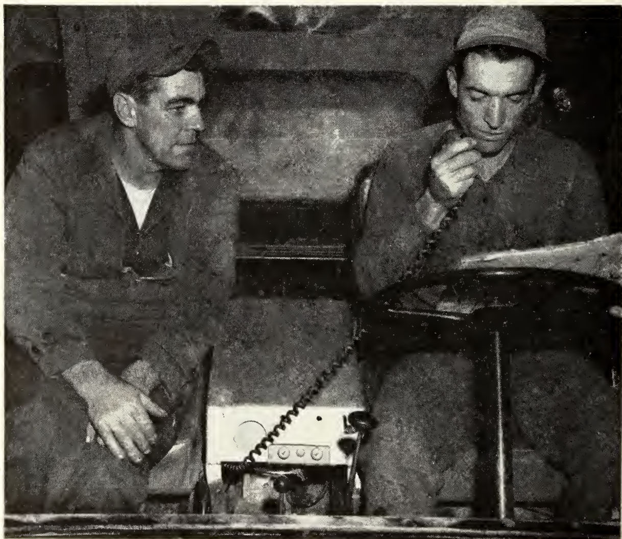
FIGURE 1.—FM radio mounted between front seats of a 1/4-ton jeep.
