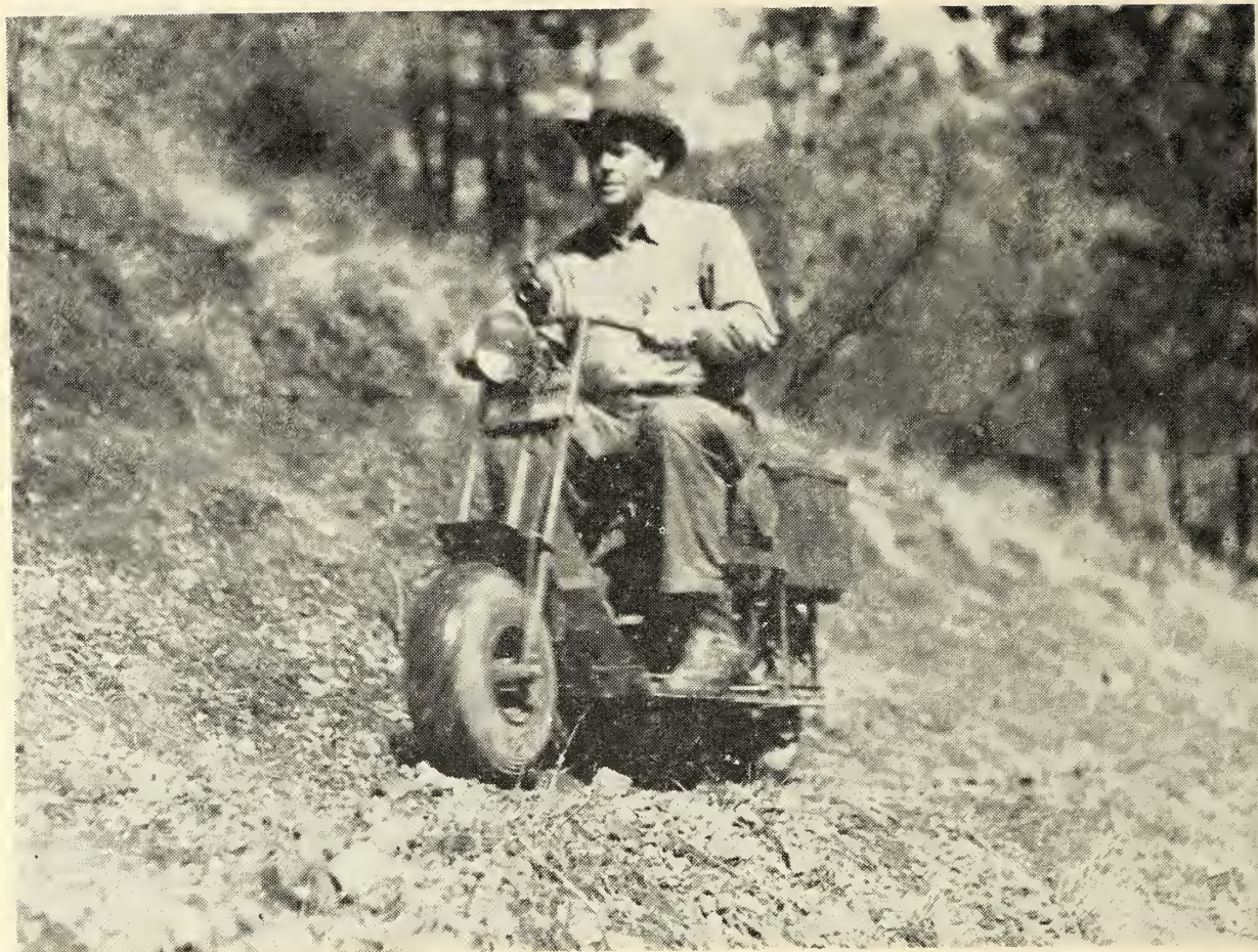
FIGURE 2.—The trail scooter provides rapid one-man transportation when trails are constructed on reasonable gradients.
