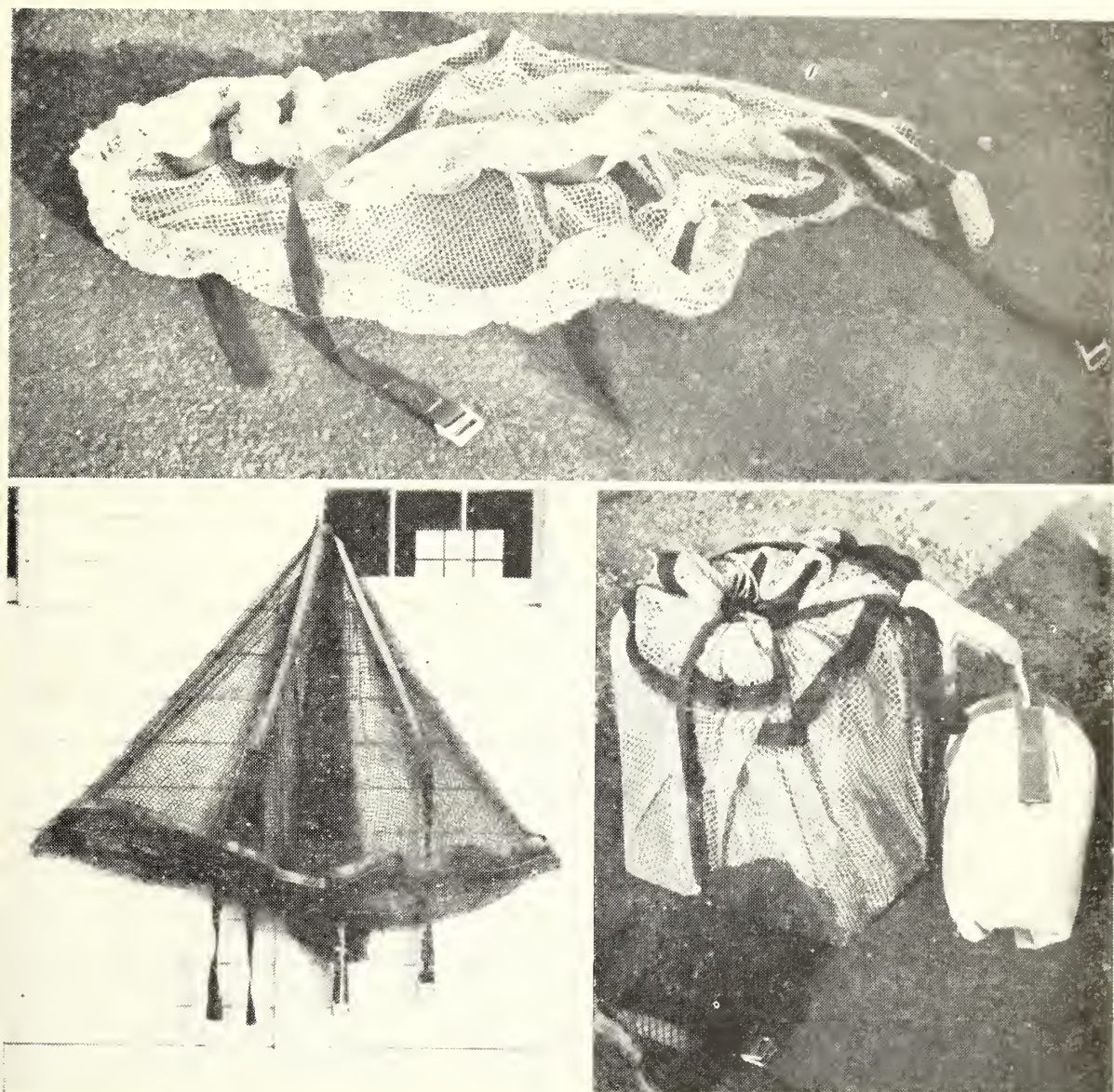
FIGURE 1.—Experimental cargo nets: new, white fish netting; inexpensive, used fish netting (dark green); white netting containing cargo and with chute attached.
