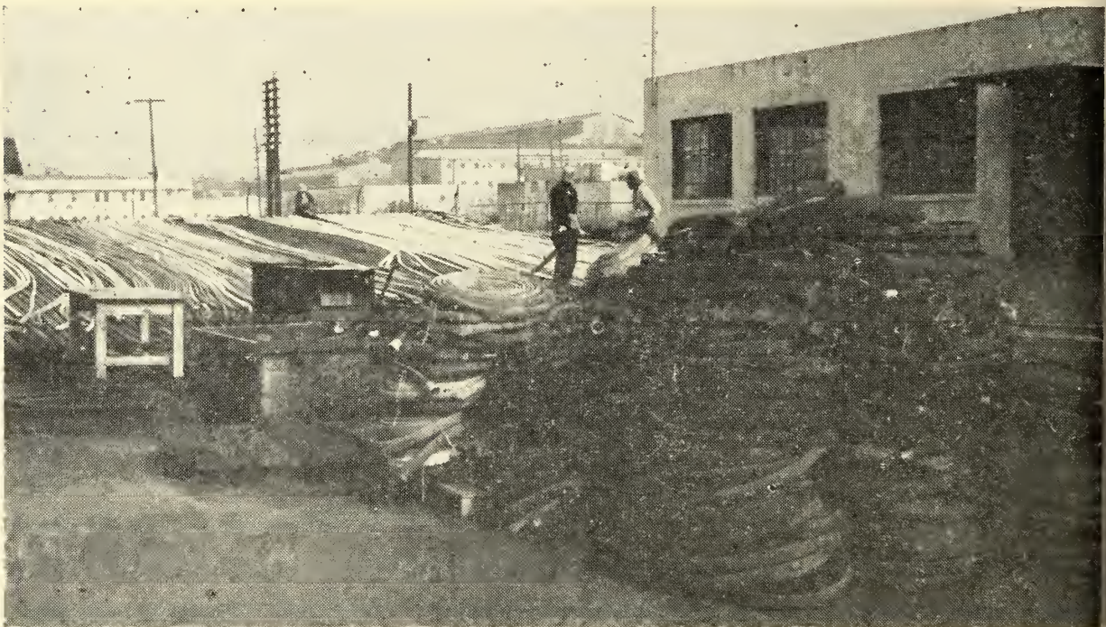
FIGURE 1.—Dirty hose in from the fires to be washed, tested, dried, rolled, and stored away. If rains persist, the hose must be dried inside. During the latter part of the 1952 fire season, 80,000 feet of hose and 52 pumpers were shipped from the Portland fire cache.
