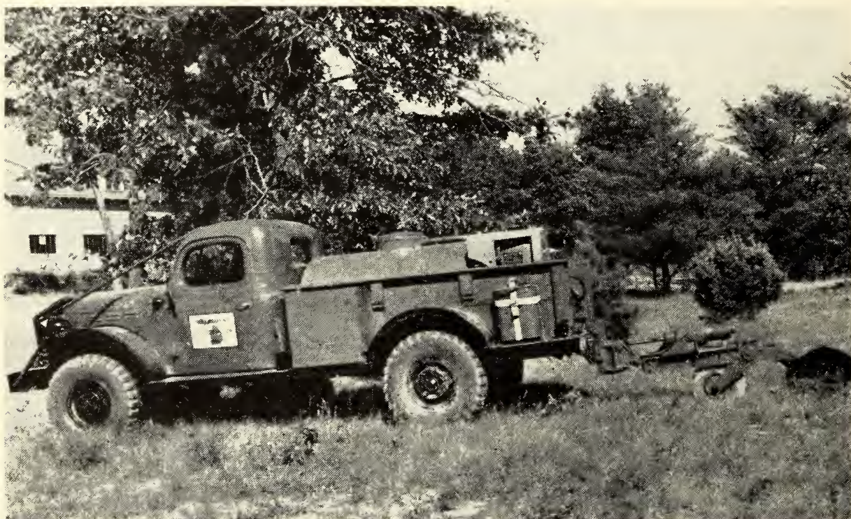
FIGURE 1.—Michigan power wagon with hydraulically controlled fire line plow ready for use.
