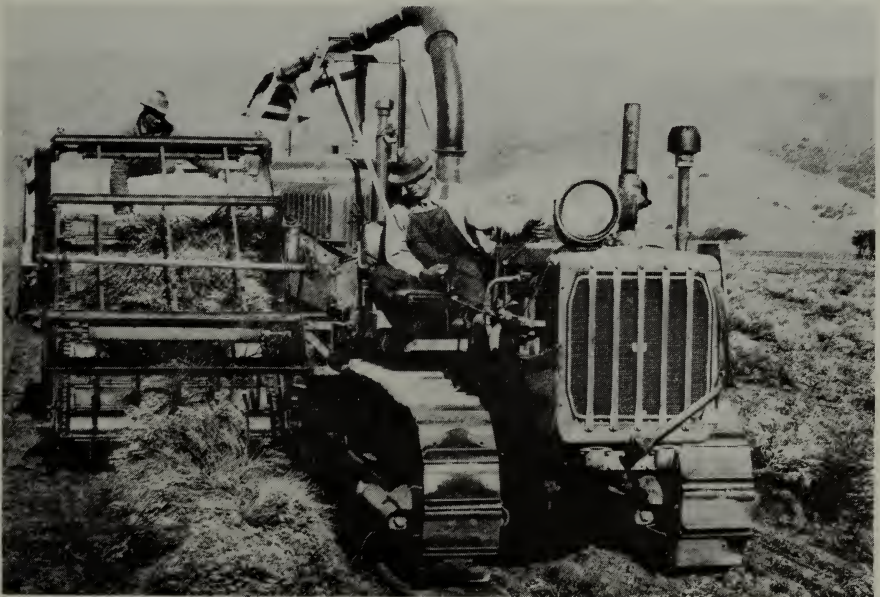
Fig. 9. At the time of the Second World War, cultivated stands of guayule shrubs were already being harvested by mechanical means. The machine harvester shown here is picking up the guayule shrubs, and chopping and loading them onto a truck bed. (Photo: National Archives)
