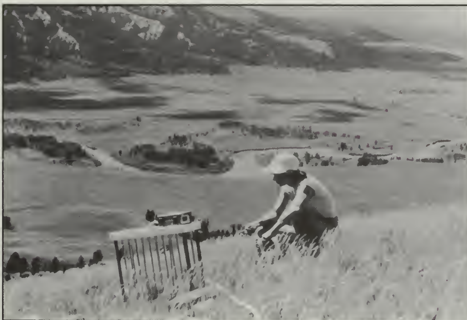
Figure 17.1 Capacitance meter used for sampling green herbaceous phytomass on Mount Norris, northeastern Yellowstone National Park.
