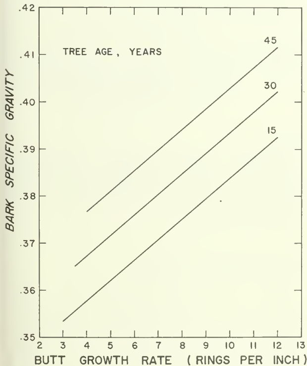
Figure 10.—Tree-average bark specific gravity as related to tree age and growth rate at butt.
