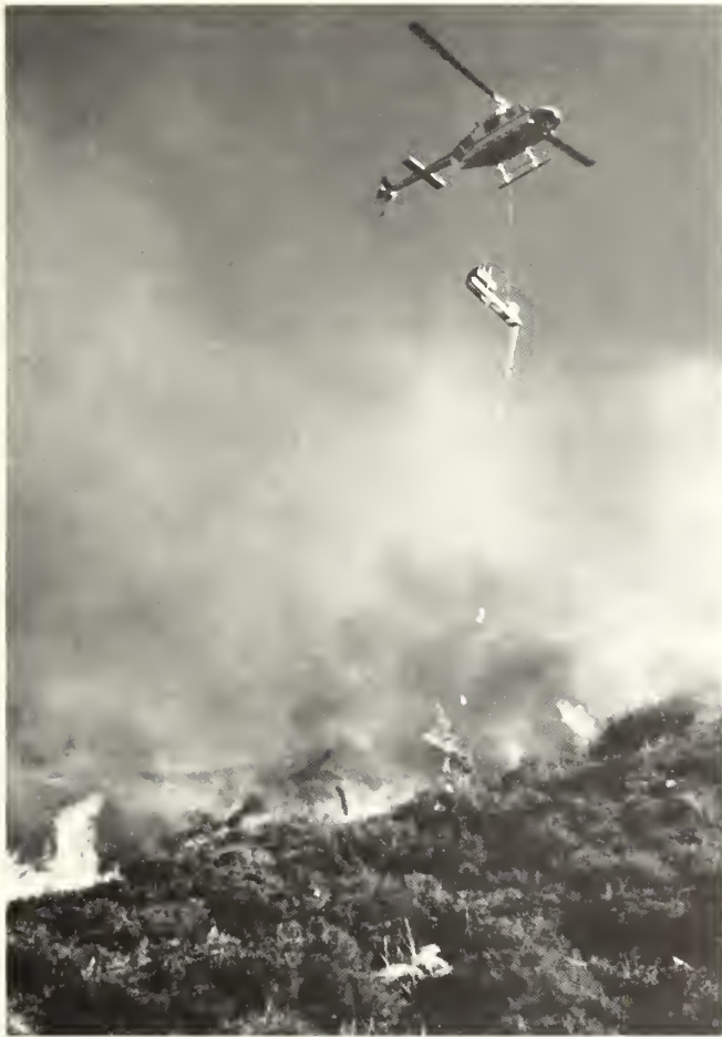
Figure 5 —The helitorch drops flaming globules of jellied gasoline that carries fire through the brush igniting dry sticks and leaves.
