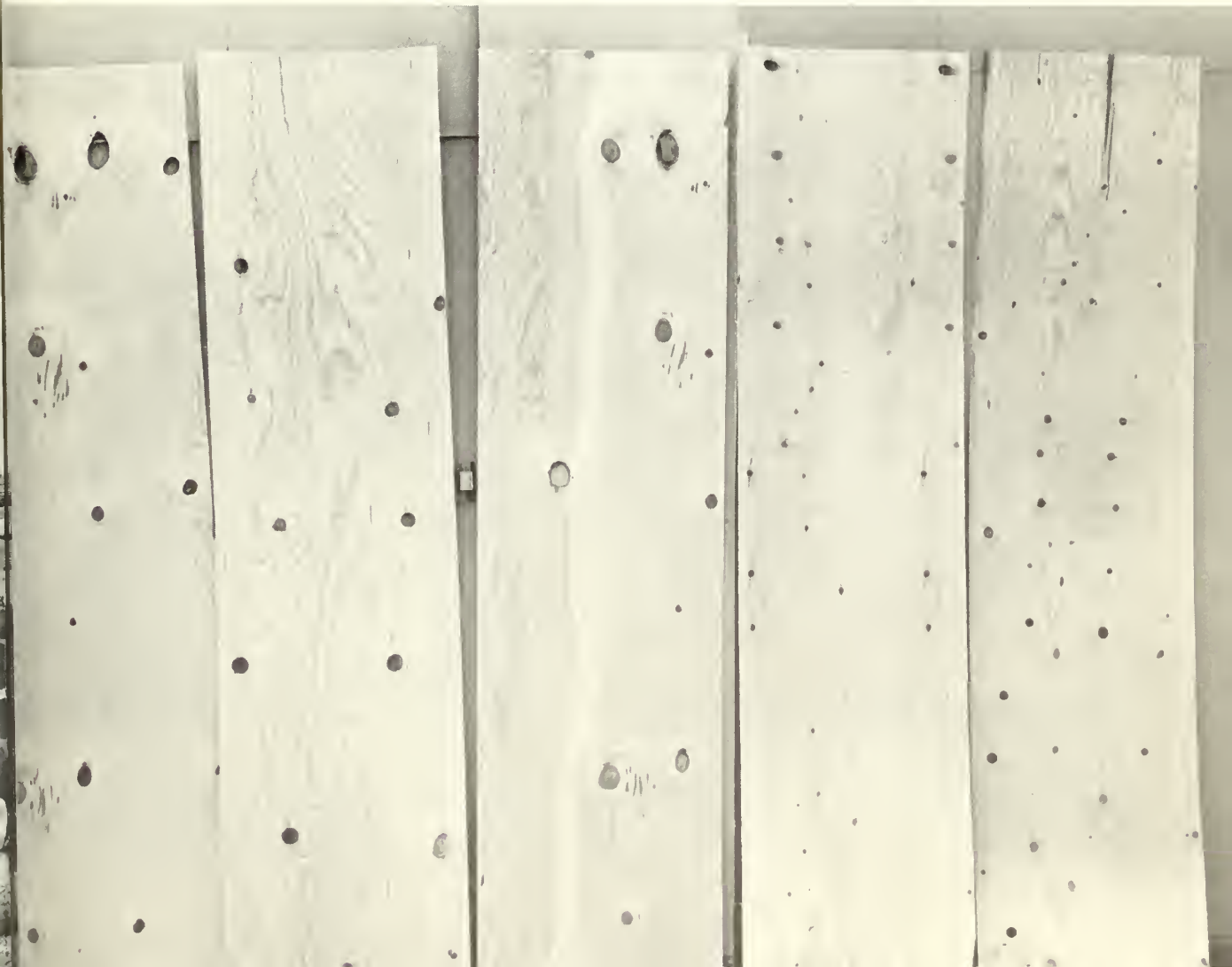
Figure 3.--Grade C veneers, represented by the two panels on the right, may have knots up to 1-1/2 inches across and holes up to 1 inch across. Grade D veneers, represented by the three panels at left, may have knots without limit and holes up to 2-1/2 inches across.
