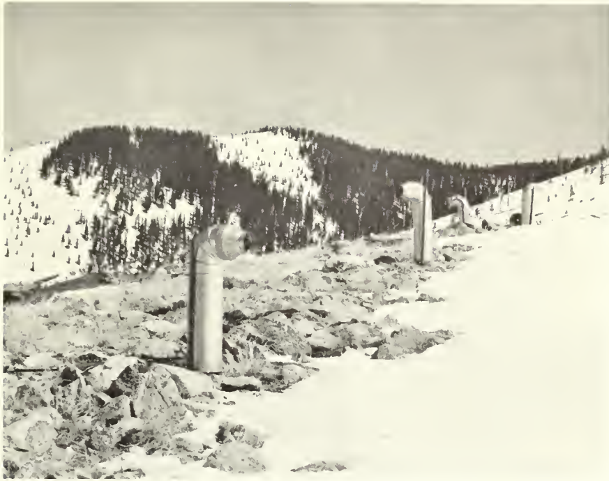
Figure 3.--Directional snow gages on an open ridgetop. Diameter of gage orifice is 4 inches.
