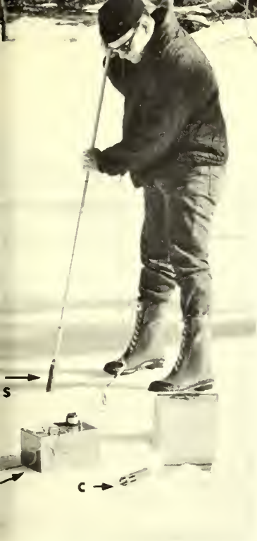
Figure 1.-- (s) temperature probe (i) Wheatstone bridge instrument (a) stainless steel cover
