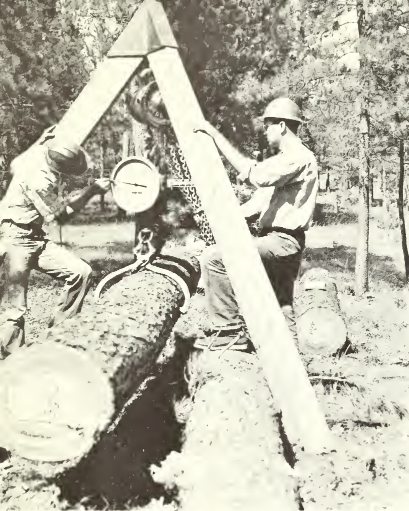
Figure 3.--Logs were weighed to the nearest 5 pounds every 3 weeks with this hydraulic load cell, chain hoist, and tripod.
