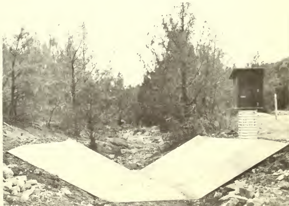
Figure 1.--A modified trapezoidal flume made with prefabricated components. Dimensions are 5 feet wide in the approach section (foreground), constricting to 1 foot in the measuring section. Sidewalls are at 30° from the horizontal, and the flume is on a 5-percent slope. Depth is 3 feet, accommodating a maximum discharge of 222 cfs.
