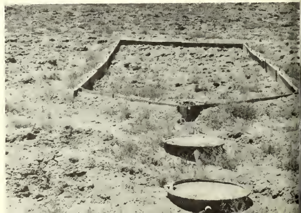
Figure 13.-- Wood border banked with soil on outside proved the most effective. Note the V-shaped collection trough.
