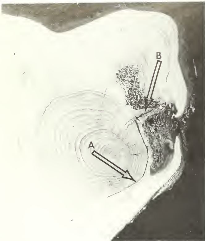
Figure 11.—Wood in the butt of A. balsamea did not decay into the central discolored wood or outward into the wood that formed after the infection. A ring shake (arrow A) was associated with a barrier zone from an old wound. Arrow B shows the radial shake associated with the old wound. Note that the decay associated with A. mellea did not develop in the discolored wood around the radial shake. The faint discolored areas in this sample were associated with the tops of other columns of decayed wood associated with root infections.
