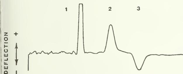
Figure 1.—Polarimetric deflection of the monoterpene olefins of a fungal lesion of loblolly pine after resolution by HPLC. (1) alpha-pinene (321  $\mu$ g); (2) beta-pinene (207  $\mu$ g); (3) limonene (57  $\mu$ g). Optical rotations were measured at the Hg, 302 line. (Note that at this wavelength ( $\alpha$ )-alpha-pinene and ( $\beta$ )-beta-pinene read positive, while ( $\gamma$ )-limonene reads negative.)
