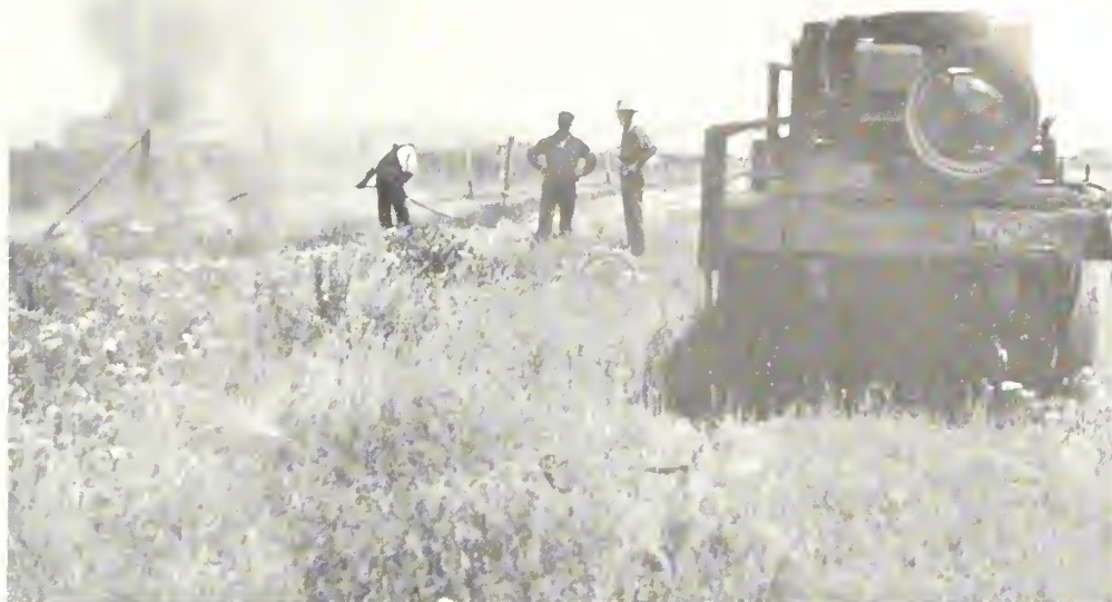
A 3-horsepower spray pump operating 1 to 3 burners and spraying 5 to 6 gallons per minute
