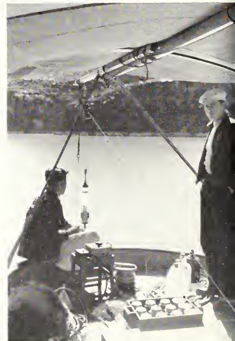
Taking water sample which shows division line between a silty underflow and clear water
