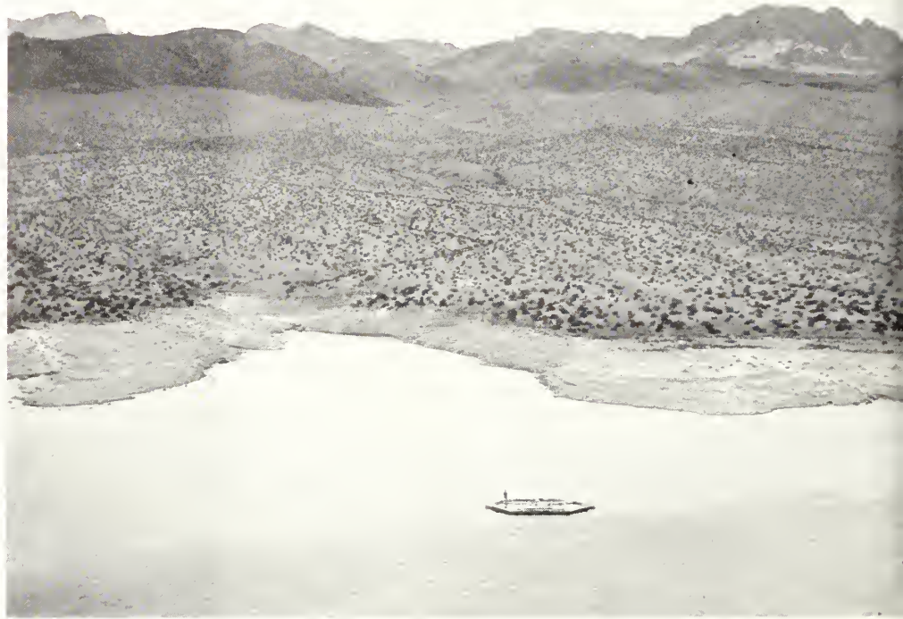
No. 2.—Floating evaporation pan on the south side of the Las Vegas Wash. In center within white fence is the Nevada land evaporation pan
