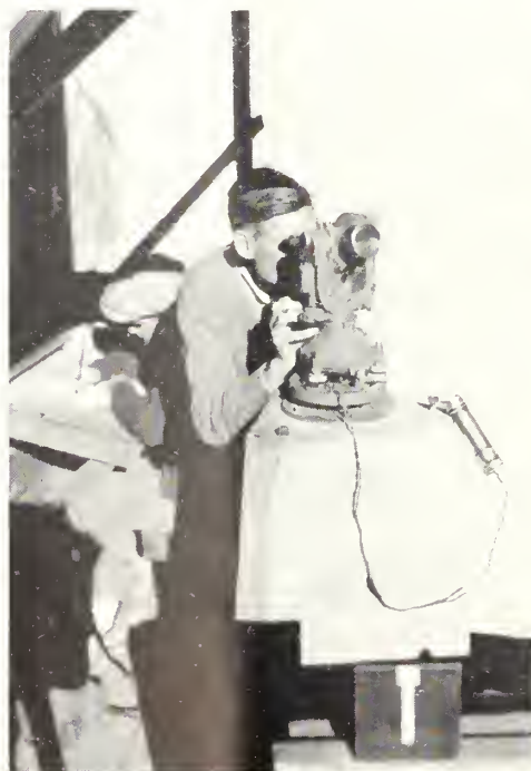
Wilde theodolite being used to observe canyon wall targets, one of the procedures in obtaining deformation of downstream face of the dam
