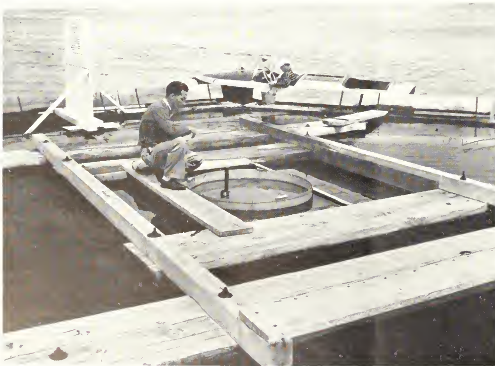
No. 1.—Technician prepares to measure evaporation in pan
