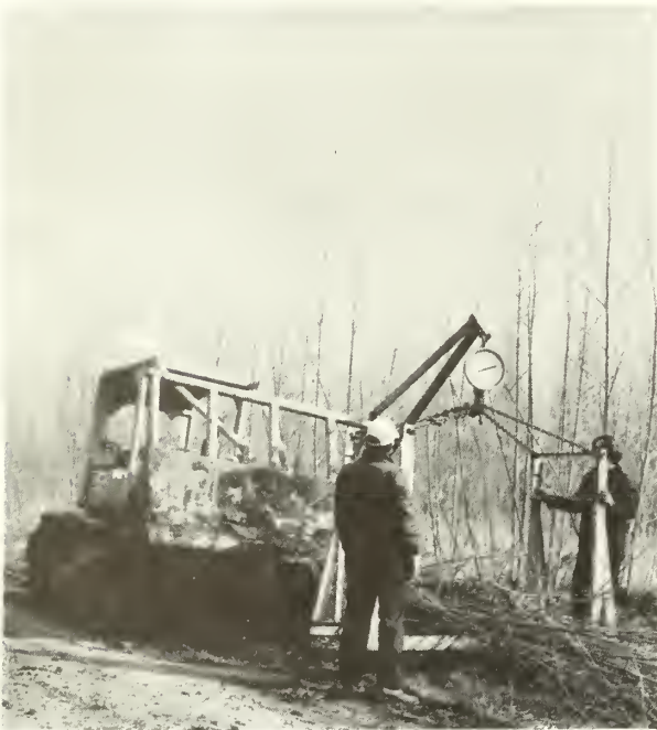
Figure 1 —Weighing freshly cut green trees at the plantation site
