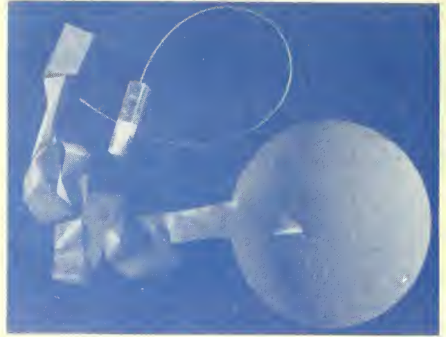
Figure 2.— Nerf ball radio transmitter package.
