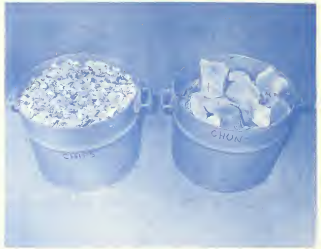
Figure 1.—Test setup for natural convective drying of chips (left) and chunks (right).
