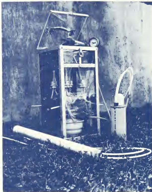
Figure 4.—Completed CCWCI with ceramic soil water samplers and small hand-held vacuum pump.
