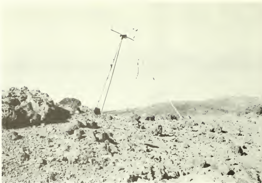
Figure 2.--Wind vane and anemometer installation at station C.
