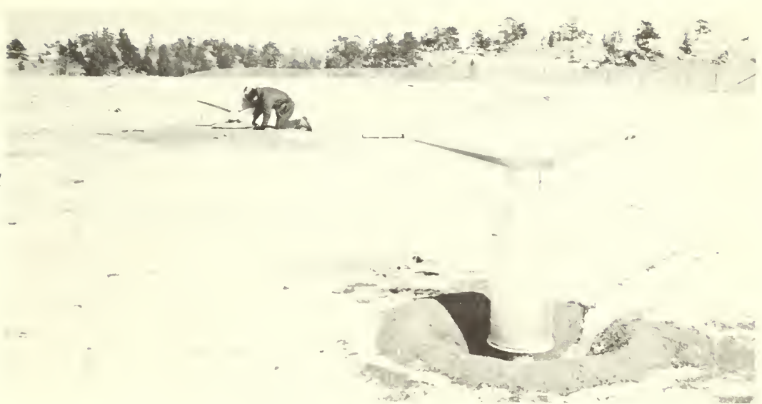
Figure 6.-- Blowing-snow gages installed with orifice heights of 1 and 0.5 meter above ground.
