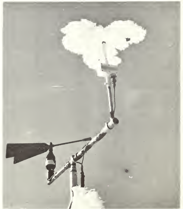
Figure 1.--Soft rime accumulation on the unheated, three-cup anemometer at the Colorado site.
