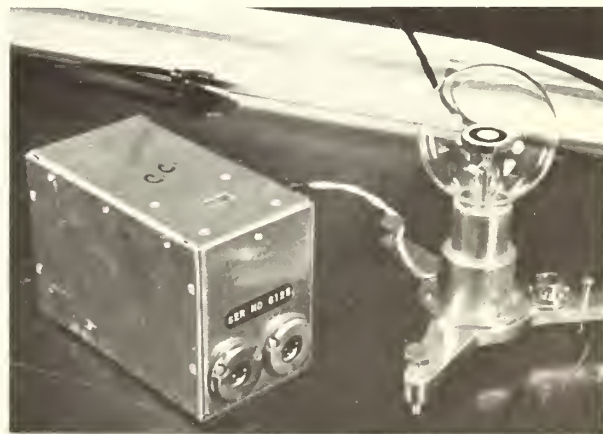
Figure 1.--Voltage integrator sums millivolt signal from pyranometer directly in langelys and displays it on a 5-decade counter. It can be read over any time period of interest from 5 minutes to several days.
