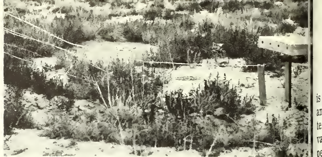
Figure 1.--Temperature sensing bulb was suspended 1 foot above bare ground under highly reflective sheet metal cover. San Luis watershed III.
