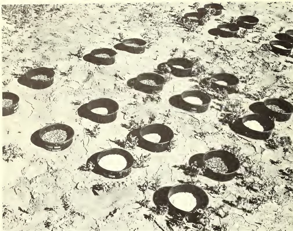
Figure 1.--Shown are three of the four replications of eight treatments used in the study. Collars are about 3 inches above the ground and 1 inch in the ground.
