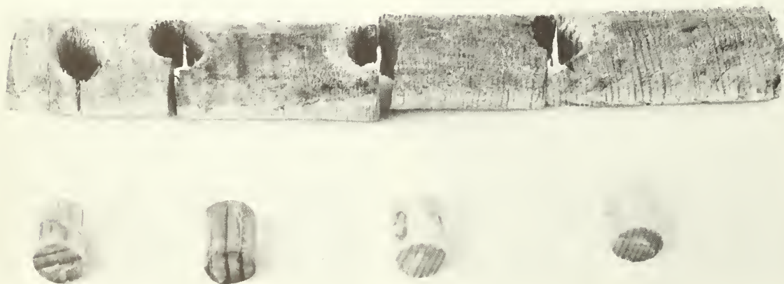
Figure 1.—Four permeability specimens cut from an increment core.
