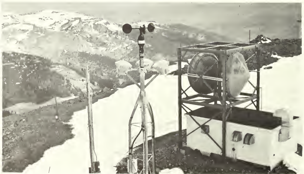
Figure 2.--Electric infrared de-icer and cup anemometer on the 12,493-foot summit of Colorado Mines Peak. The unit performed well during winters 1968-69 and 1969-70.
