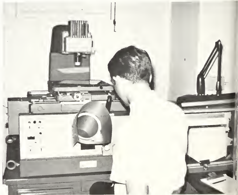
Figure 15—A microdensitometer (General Aniline and Film Corp. Model 650) was used to measure point-sample image density values of the various plant community systems. The operator is aligning the ERTS sample cell in the view screen before reading the apparent optical image density.
