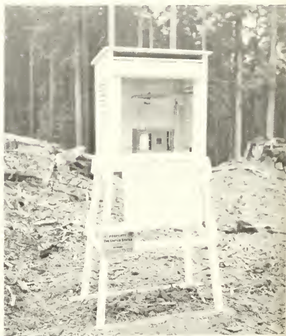
Figure 1—Soil-related temperatures were measured with this simple supporting device which holds maximum and minimum bulbs at the surface, as well as 1 inch below and 1 inch above the surface ( left ). Ambient air temperatures were measured in a standard Weather Bureau-type shelter ( right ).
