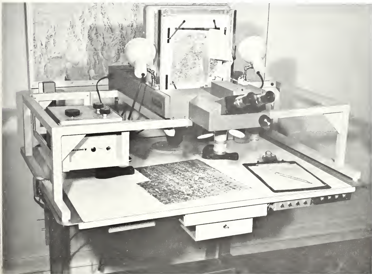
Figure 5—Optical equipment used in photointerpretation varied with the aim of the test. Above , for land-use determinations, interpreters used an Old Delft stereoscope to view simultaneously the center point of each test sample unit on the overlay and the corresponding points on April-October and April-June combinations of ERTS color composites. Below , to locate forest disturbances, interpreters used a Bausch and Lomb Transfer Scope to view simultaneously the ERTS scene for April 1973 and the 1:63,360-scale photo index sheet for February 1966.
