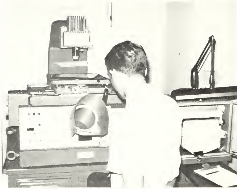
Figure 13—A microdensitometer (General Aniline and Film Corp. Model 650) was used to obtain optical image density. The photograph on the moveable image-holding stage is scanned by the light beam tube. The operator aligns the Skylab sample cell in the view screen before reading the apparent optical density registered on a digital display. The viewing screen and stage also aided in the estimation of foliar cover from large-scale photos.
