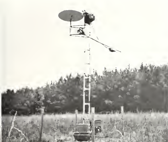
Figure 24—Instruments and equipment for the data collection experiments were set up at four sites within sub-block 2. Shown at the top of the tower ( left ) are the data collection platform (DCP), antenna, incident-energy spectrometer, multiplexer, and light-activated switch. At the end of the 4-m boom arm is the reflected-energy spectrometer. Alkaline battery power packs are at the base of the tower. The interior of a field spectrometer is shown at right .
