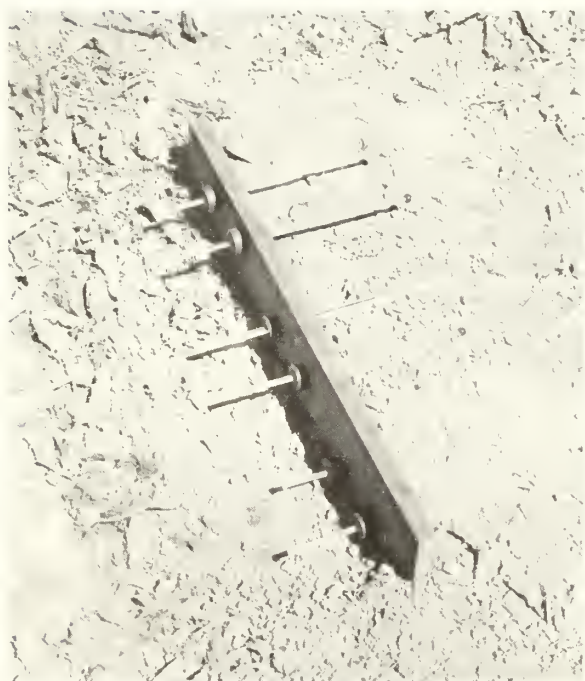
Figure 1—Soil-related temperatures were measured with this simple supporting device which holds maximum and minimum bulbs at the surface, as well as 1 inch below and 1 inch above the surface ( left ). Ambient air temperatures were measured in a standard Weather Bureau-type shelter ( right ).
