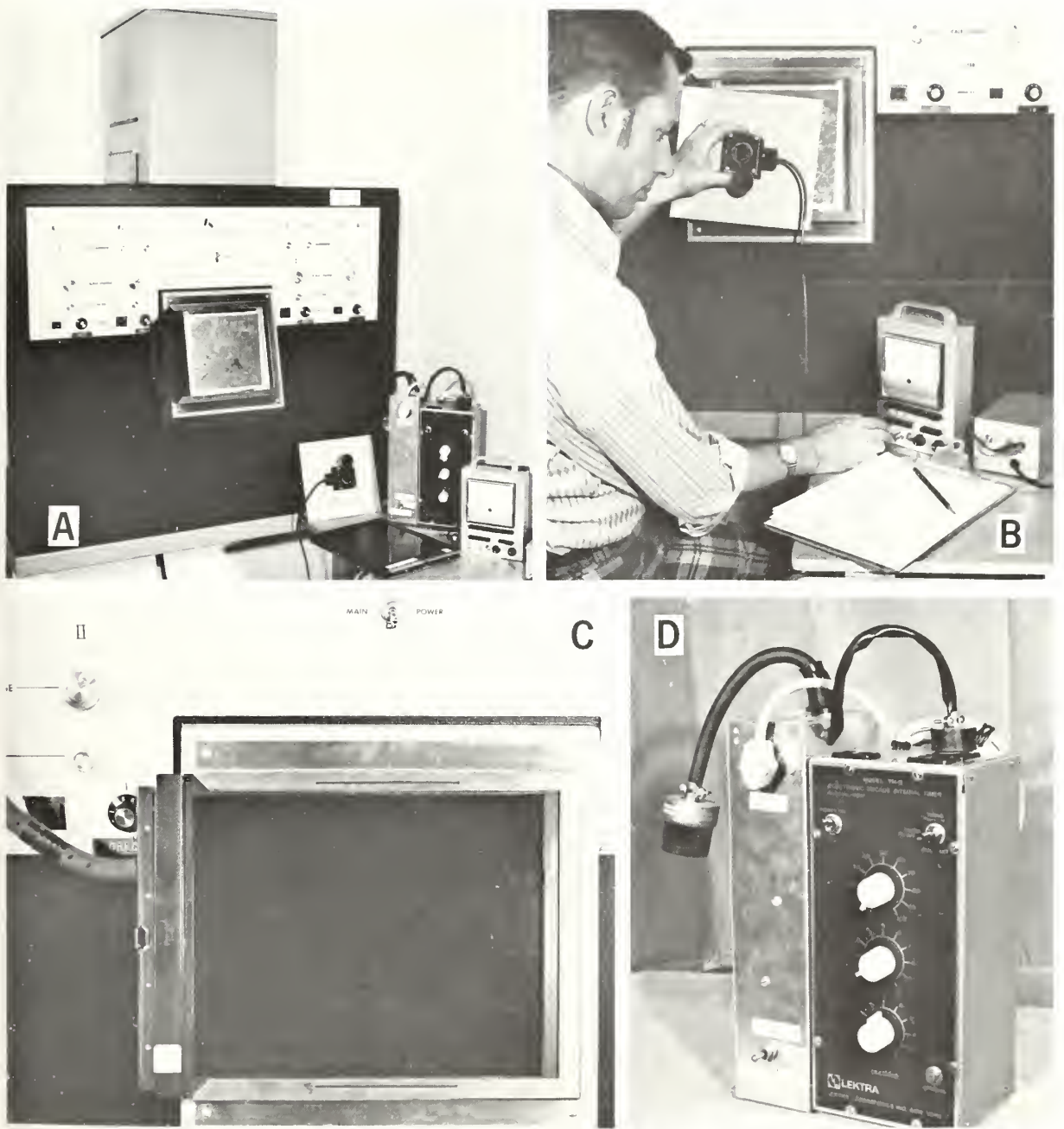
Figure 29—Equipment required to make color internegatives from ERTS 70-mm transparencies included (A) I 2 S additive color viewer with photometer and high-speed timer, (B) Forest Service-designed photometer used to measure light intensity of each MSS band and of the color composite, (C) 8 by 10-inch vacuum film holder (vacuum hose, left ), and (D) Lektra decade interval timer ( right ) with heavy-duty relay and switching circuit box ( left ).
