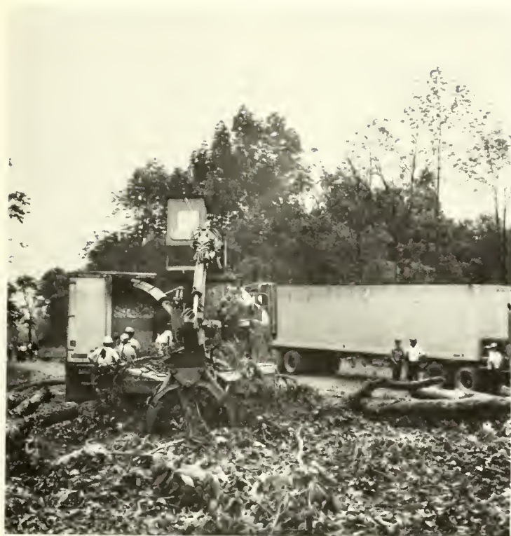
Whole-tree chip harvesting has enabled operators to use smaller trees, tops, branches, and other nongrowing stock sources to meet wood requirements.
