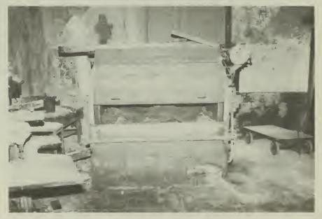
Front view- "Smith Drum", right side dial is numbered to "60" and operating buttons are labeled: "STOP-INCH UP" and "STOP-INCH DOWN".
