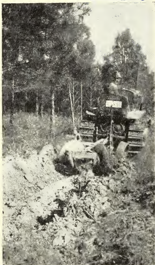
Fire-line plowing with 40 H.P. tractor and 3-disc Hester plow in southeastern Louisiana
