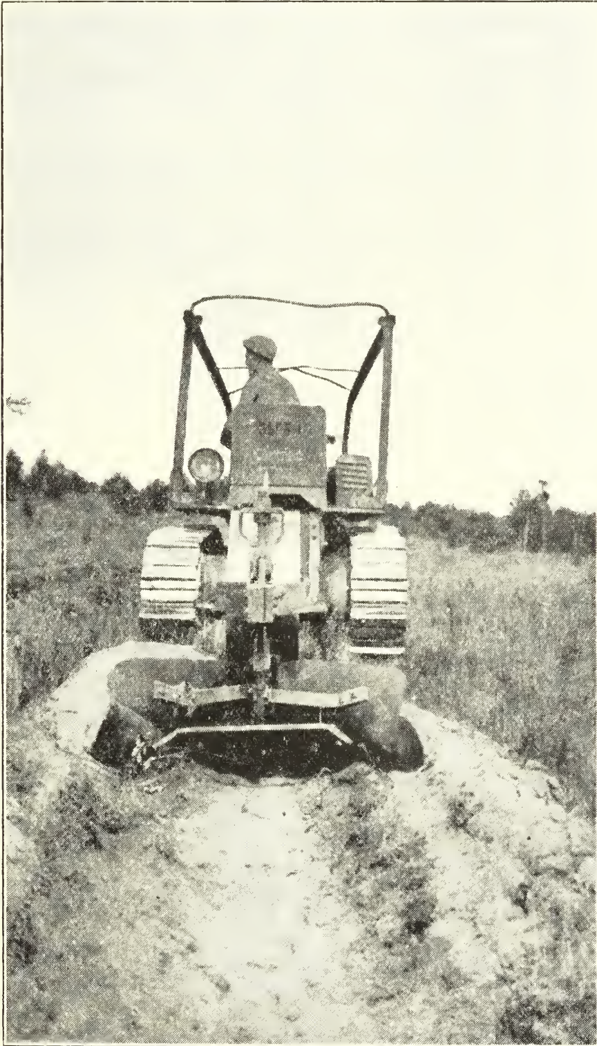
Fig. 5—Type of furrow produced by plow. Action is very similar to Killefer 77. In this particular type of plowing the Killefer 77 cannot be drawn faster than in second gear. This plow will travel in high. The picture also shows construction detail of moldboard assembly from rear. Stability is indicated in this picture.
