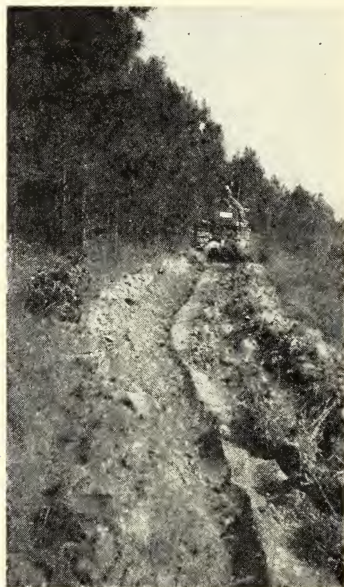
Fire-line plowing with 40 H.P. tractor and 3-disc Hester plow in southeastern Louisiana
