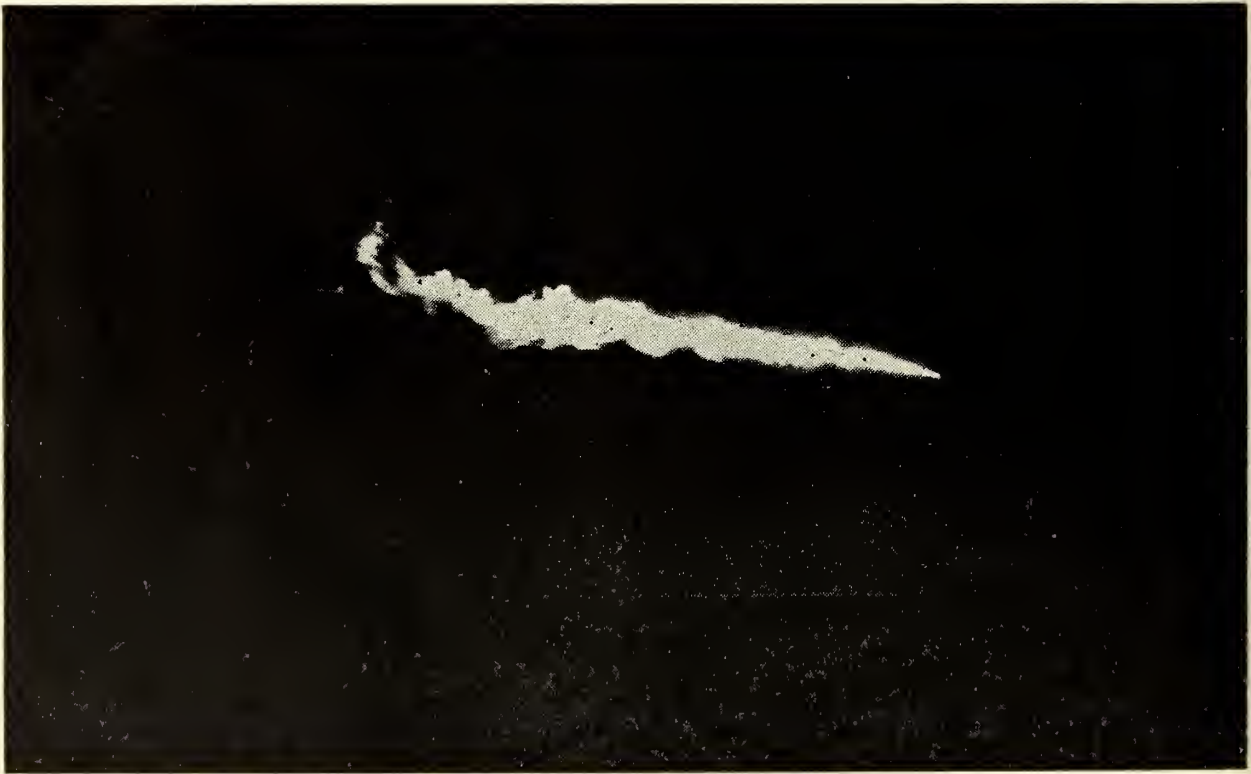
Flame produced by the flame thrower on the pressure stroke of the pump. Distance from camera—40 feet.
