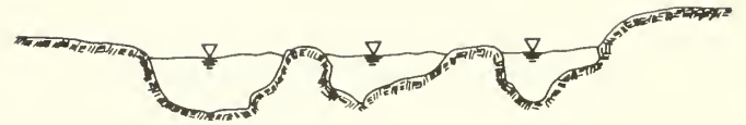
Figure 19.—Schematic diagram of a channel cross section in an anabranching river. The overall appearance suggests several independent parallel streams.
