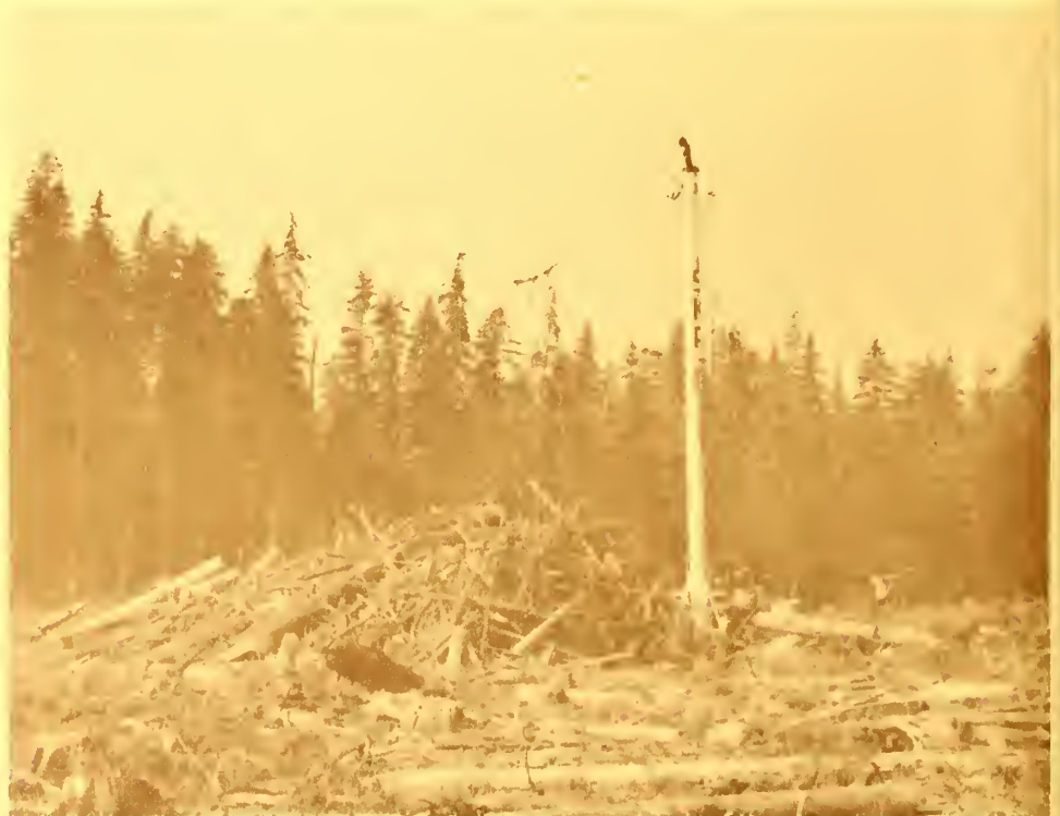
Figure 1.--High-lead tower yarding to residue pile on Unit 1, Trout Creek Hill timber sale.
