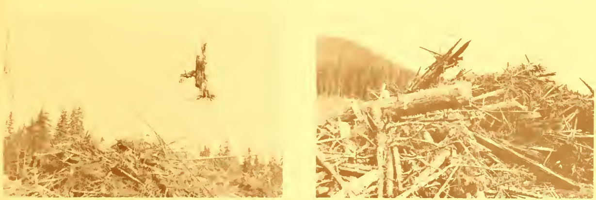
Figure 2.--Two turns of residue material being yarded to piles on landing.
