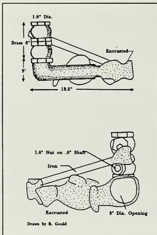
**Figure 18.4.** Valve assembly. Drawing by Richard A. Gould.
