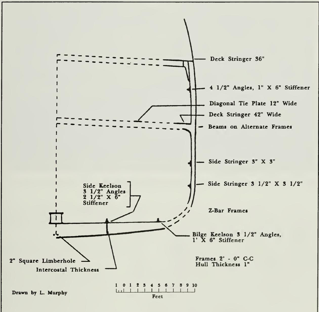
Figure 13.4. Compiled midships hull cross section.
