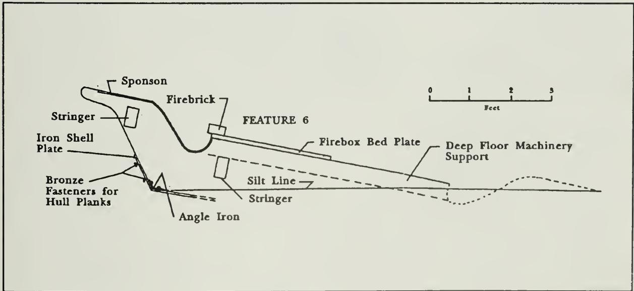
Figure 18.2. Hull cross section. Drawing by Richard A. Gould.
