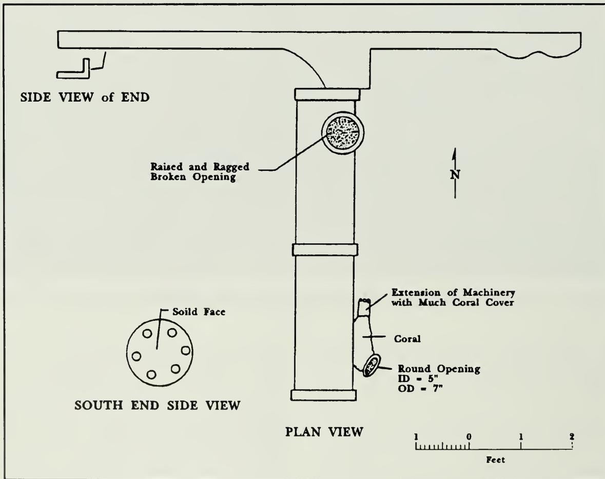
Figure 13.6. AVANTI steam machinery. Probably from a cargo winch. Drawing by Jackie Koening and Pam Krim.
