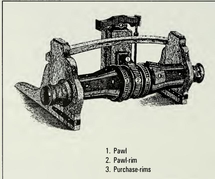
**Figure 14.6.** Drawing of wooden windlass from the midnineteenth century (after Paasch 1890:Plate 70).
