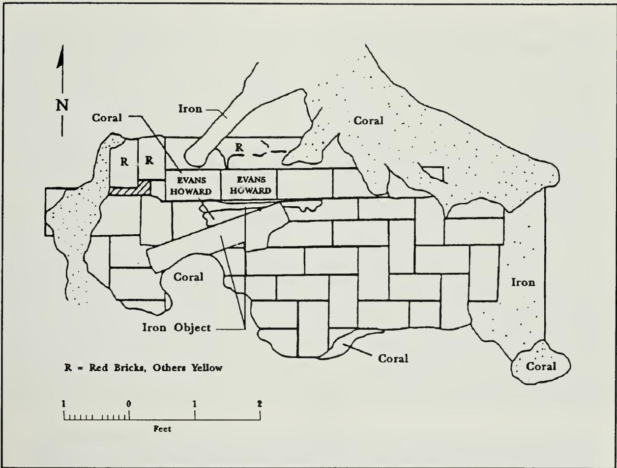
**Figure 18.3.** Brick arrangement in boiler firebox. Drawing by Richard A. Gould and Charlotte Taylor.
