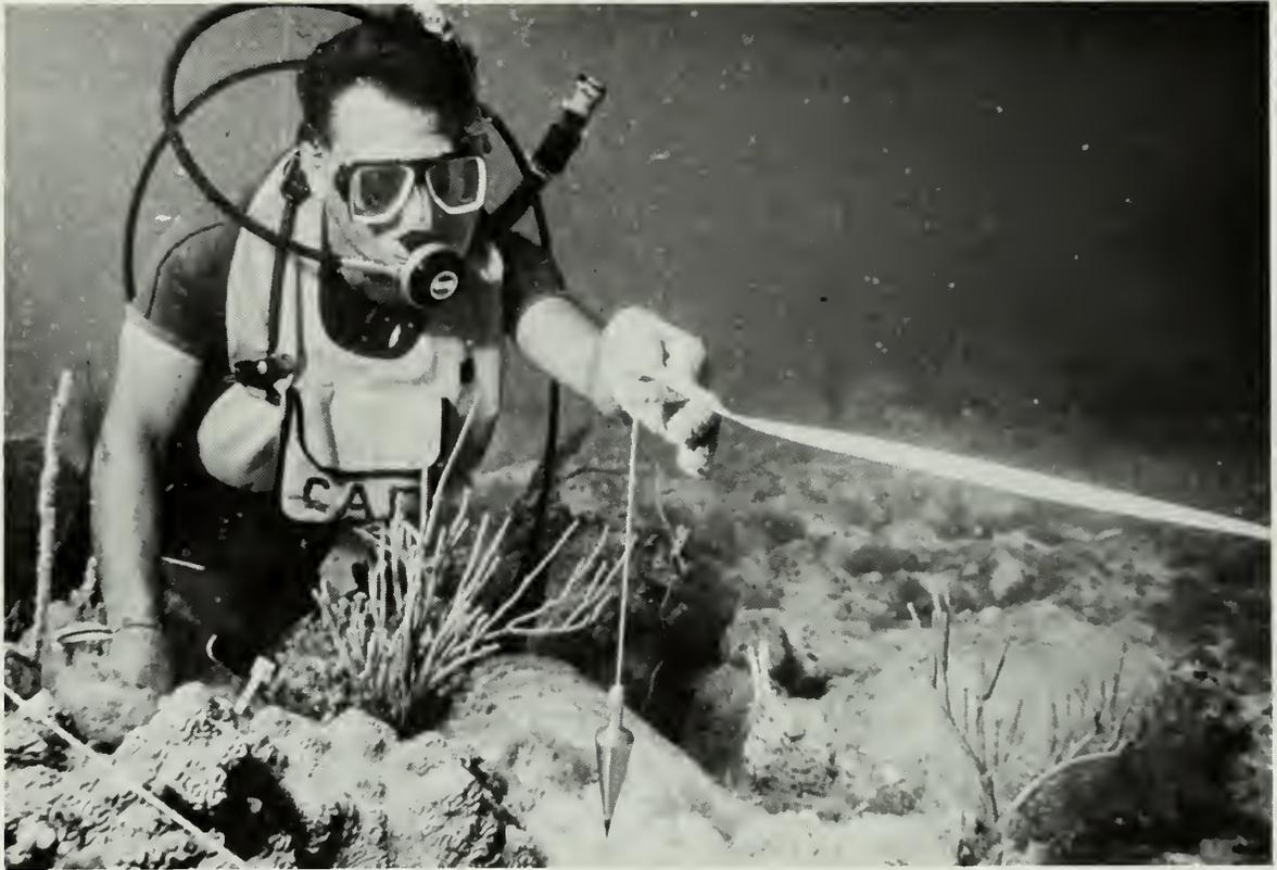
**Plate 11.7.** Volunteer Joseph Los holds a plumb-bob over a point during mapping operations. Mapping methodology utilized in all projects is base-line trilateration developed by NPS SCRU. Photo by John Brooks
