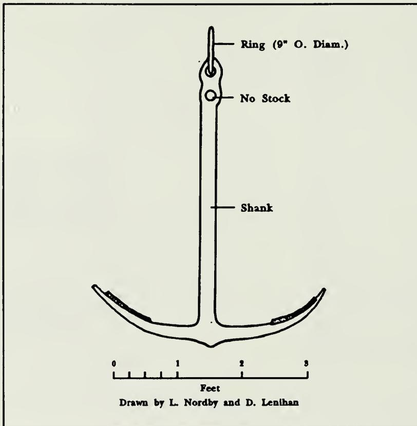
**Figure 12.7.** Anchor 2, north coaling docks. The anchor is an iron-stocked type, but the stock is missing. Drawing by Larry Nordby and Daniel Lenihan.
