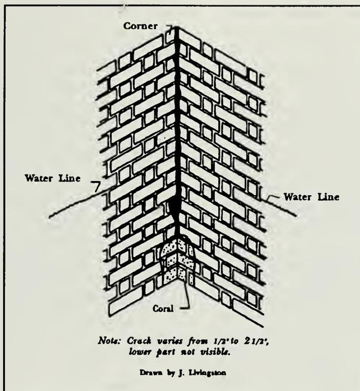
Figure 10.3. Example of 1971 wall crack survey drawings.
