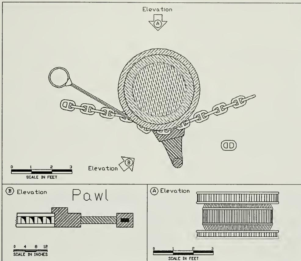
**Figure 14.4.** Capstan and stud-link chain associated with hull structure of Feature 2. Original field drawing by John Seidel; Autocad drawing by Tim Smith.
