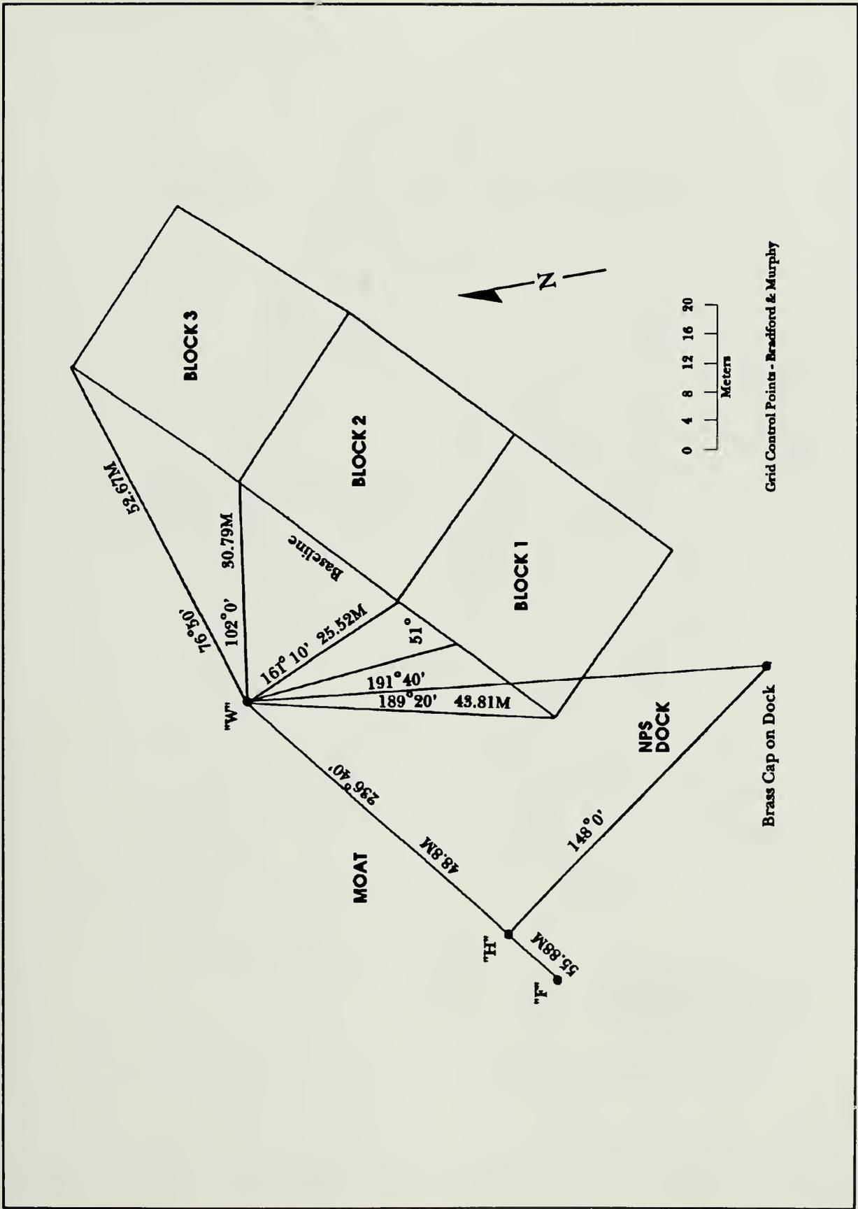
Figure 12.8. Grid control points. Drawing by Jim Bradford.
