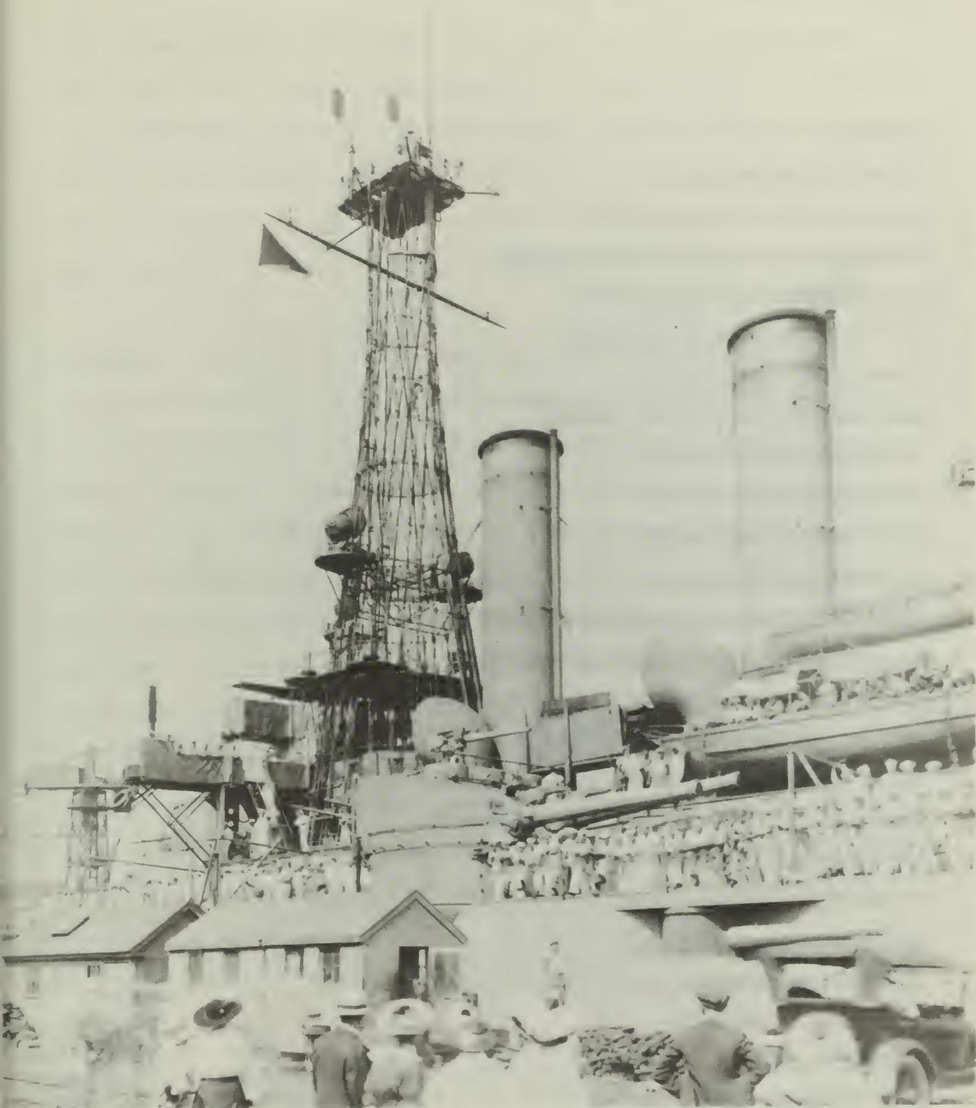
PHOTOGRAPH NO. 8: USS Rhode Island at the Boston Navy Yard, September 11, 1915. Note crew members crowding the rails and the three-inch gun mounted on top of the eight-inch gun turret.
