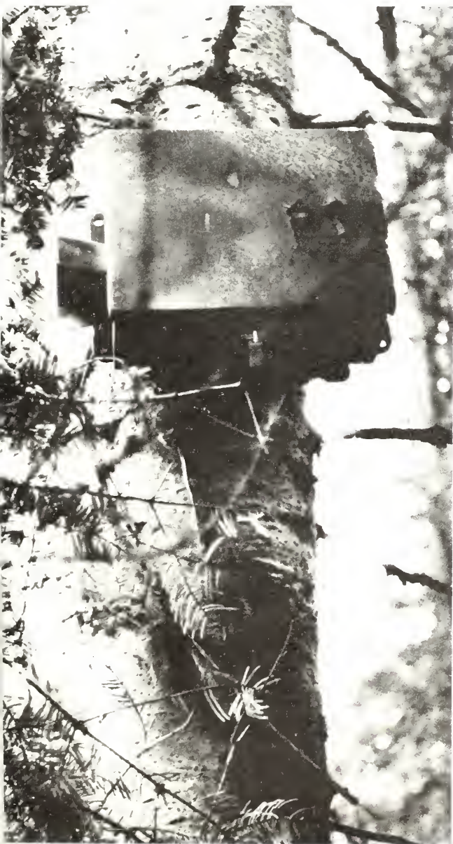
Figure 4.--Camera used to record trail traffic, mounted in a weatherproof box.
