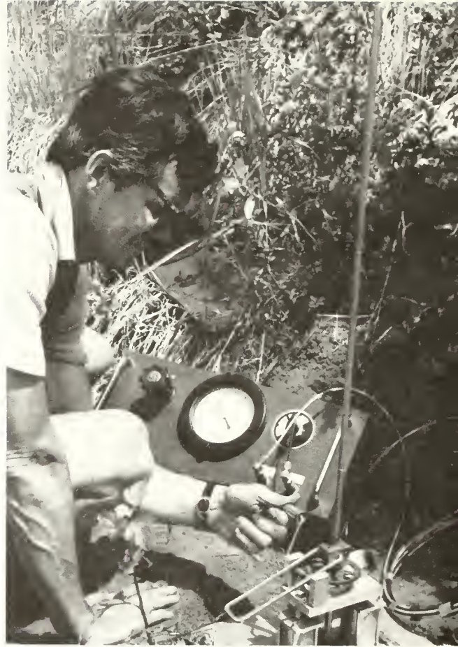
Figure 16. — Borehole, direct shear test in progress in shallow, coarse textured soil developed on granitic rocks of the Idaho batholith. Pine Creek study area, Boise National Forest.
