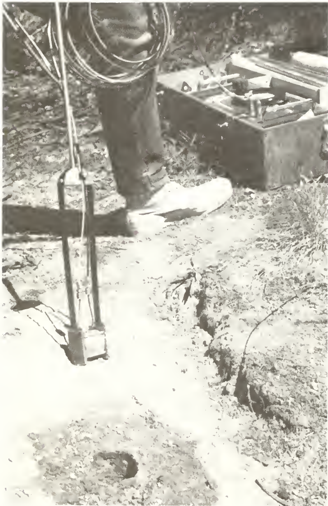
Figure 15. — Expandable shearing head of borehole device prepared for lowering down borehole.
