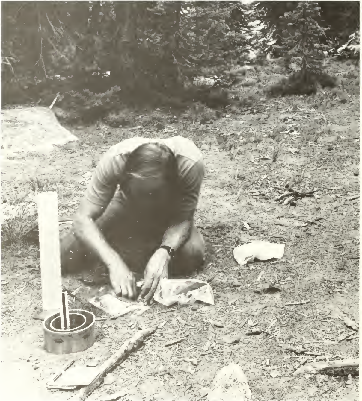
Figure 11.--Infiltration rates were measured with a double-ring infiltrometer. Soil samples were collected and the volume of the excavated hole was determined for use in calculating bulk density.
