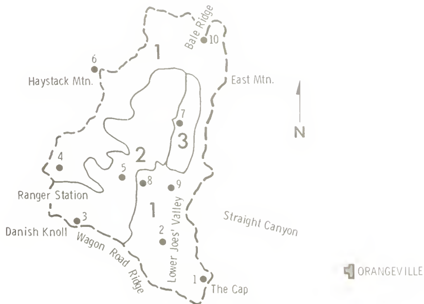
Figure 1—Map of Straight Canyon barometer watershed Utah showing zones and gauging stations.
