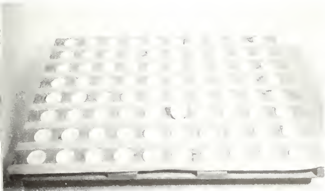
Figure 3.--Sample cup tray, one of six trays that are placed side by side and used simultaneously.
