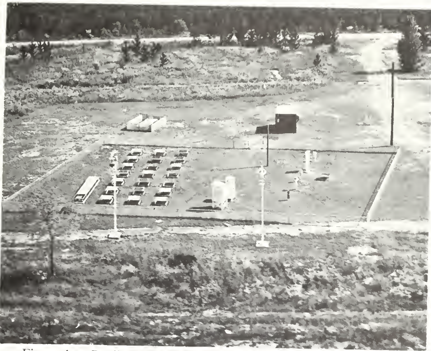
Figure 1.—Replicated stick exposures are shown at left inside the enclosure. The long frame at the extreme left held the weathering study sticks and screens. Instruments for recording the weather variables occupied the rest of the enclosure. The stick weighing shelter is shown at top right.
