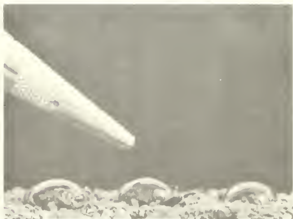
Figure 1.—Water droplets on a non-wettable soil showing their “balled-up” appearance.
