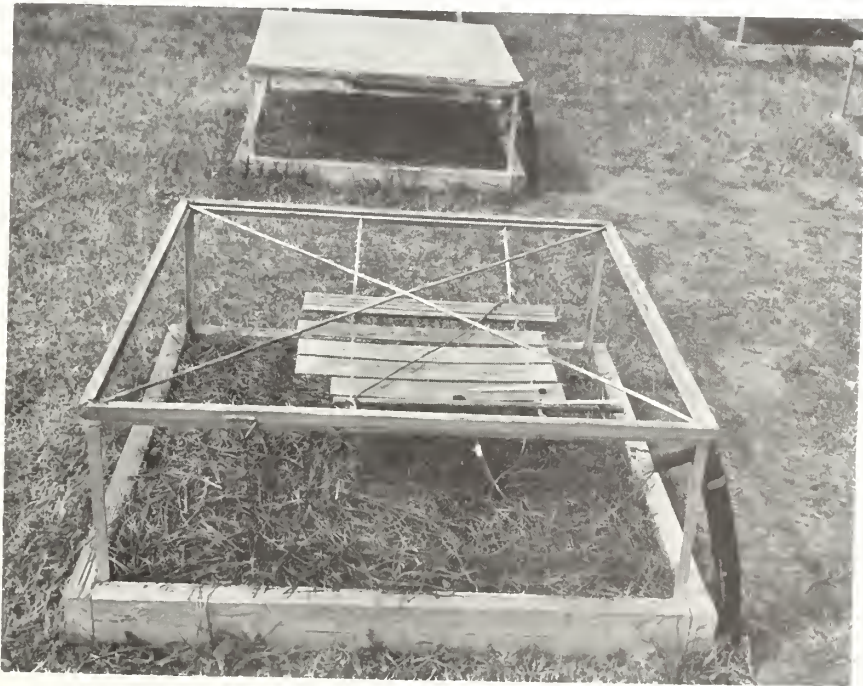
Figure 2.—Sticks exposed under no screens were placed on supports. The tube leading into the ground carried the thermocouple lead-in wires to the potentiometer in the weighing shelter. Sticks were also exposed under one, three, four, and six layers of screen.
