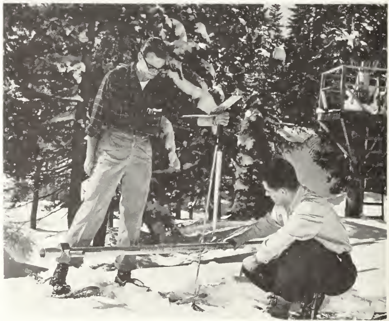
Figure 14.—Measurement of snow water at 100 special snow courses permits evaluation of management effects on water yield.
