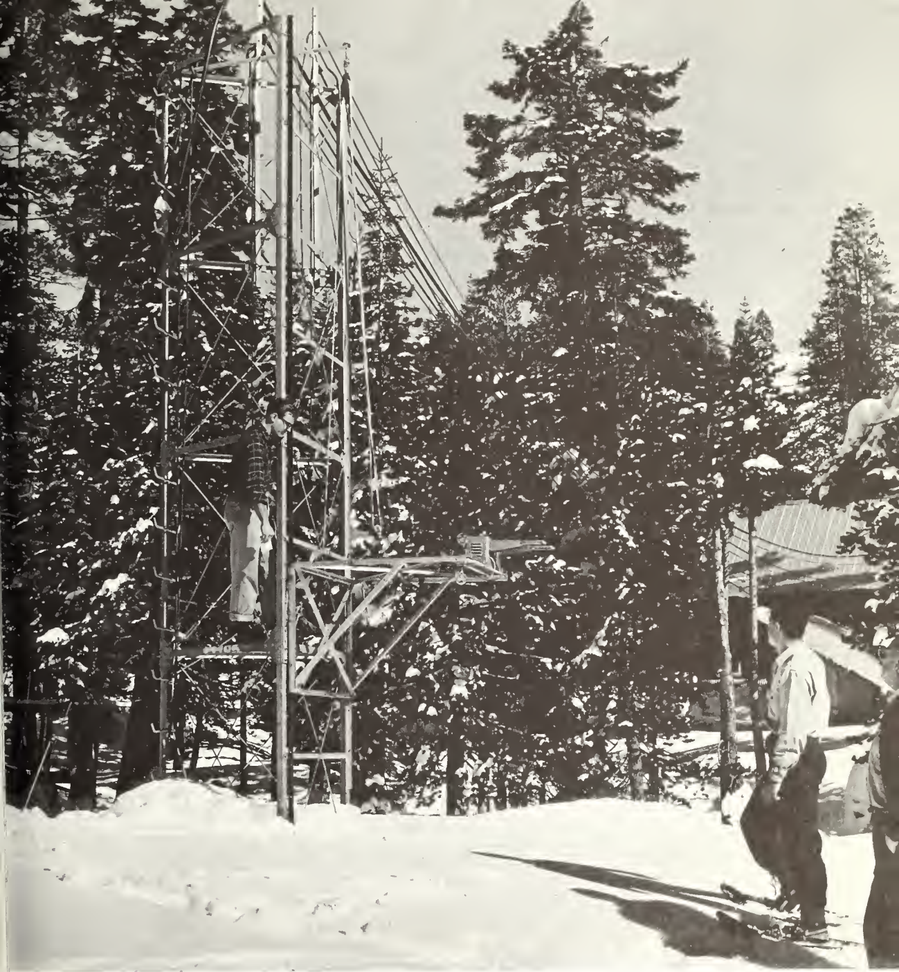
Figure 2.—Towers support meteorological instruments which help evaluate moisture losses in summer and winter, snowmelt in winter, and the effects of wind, humidity, and temperature on water losses and snowmelt.
