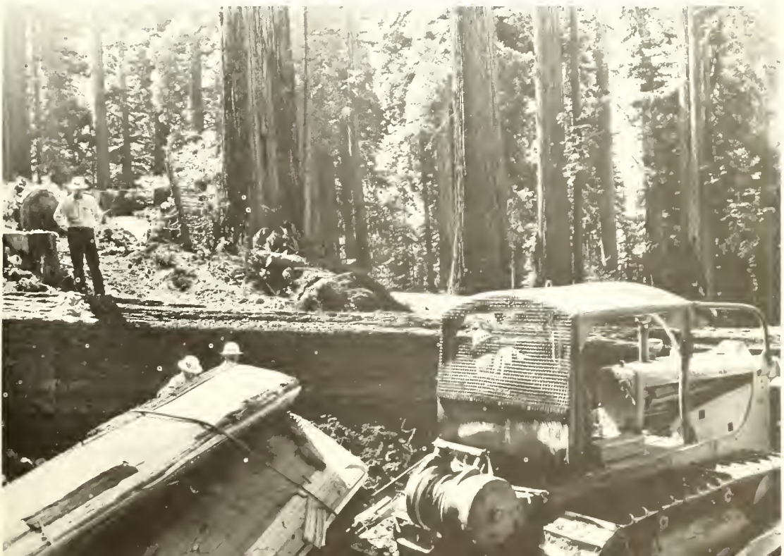
Figure 5.—Skidding production may be estimated rather accurately by the average volume per log.
