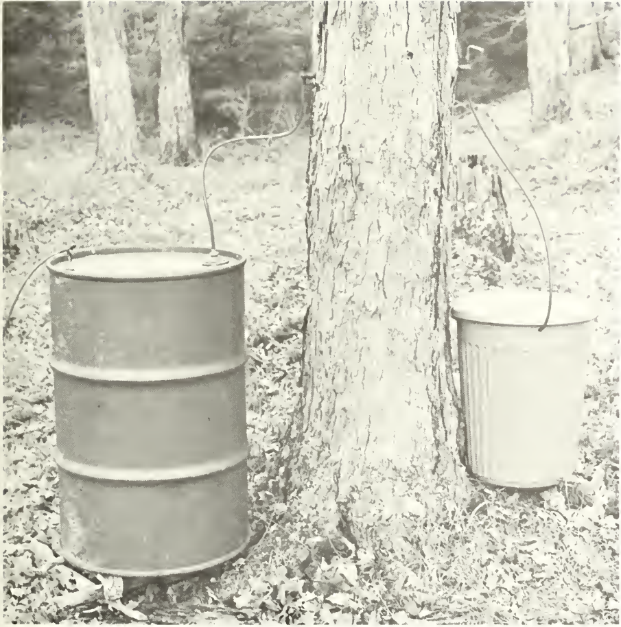
Figure 1.—Sap-volume yields were collected for each taphole, using a 55-gallon drum for the vacuum yield and a 20-gallon container for the gravity yields.
