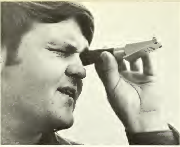
Figure 4.—Using a refractometer to measure the sap sugar concentration.
