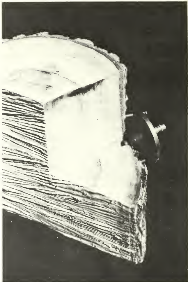
Figure 4.—Attachment of injector head. The injector head protrudes into the xylem through a hole that extends about 3 annual rings deep. The neoprene gasket is seated on bark that has been cut smooth by a 1-inch counter-bore. The injector head is nailed in place with 8-penny duplex nails.
