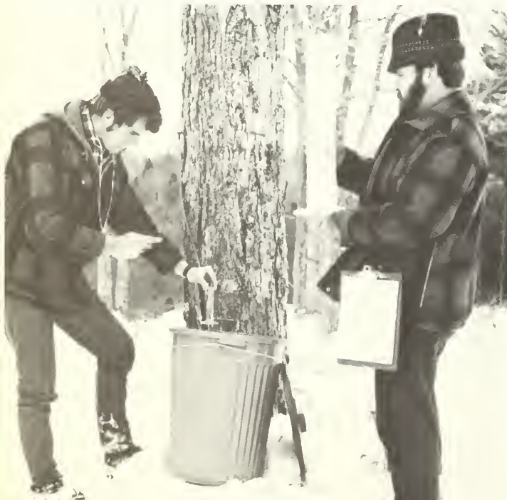
Figure 1.—Left, sap-flow rate was measured with a stopwatch and graduated cylinder. Right, sap volume was measured to the nearest ½ liter.
