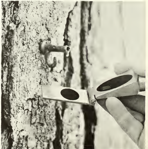
Figure 2.—A drop of sap about to fall on the dark circular area of the refractometer cover. The refractometer can be used at the tree as well as in the sugarhouse.
