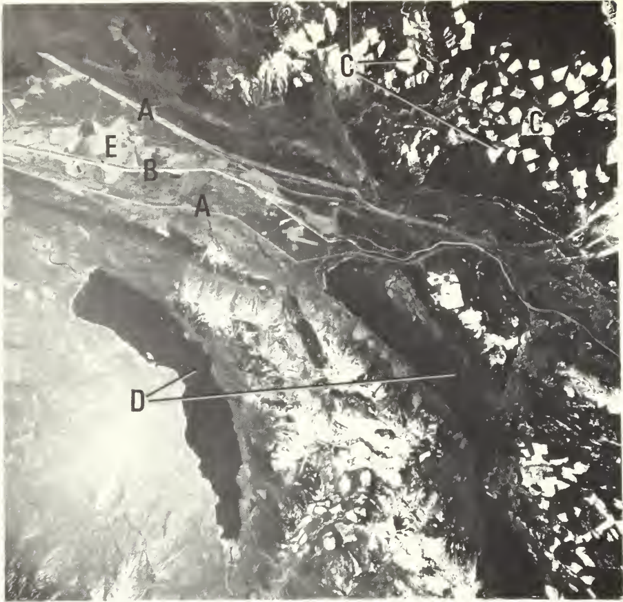
Figure 3.—Actual size of the satellite-simulated “false color” photograph printed in black and white. View is similar to the inventory area. Powerline rights-of-way (A), roads (B), logging areas (C), lakes (D), and agricultural lands (E) are easily seen without magnification. (Photo courtesy of State of Washington Department of Natural Resources.)
