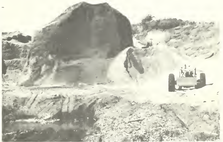
Figure 1.—Sawdust storage pile with sour center. Source of samples 1 and 4.
