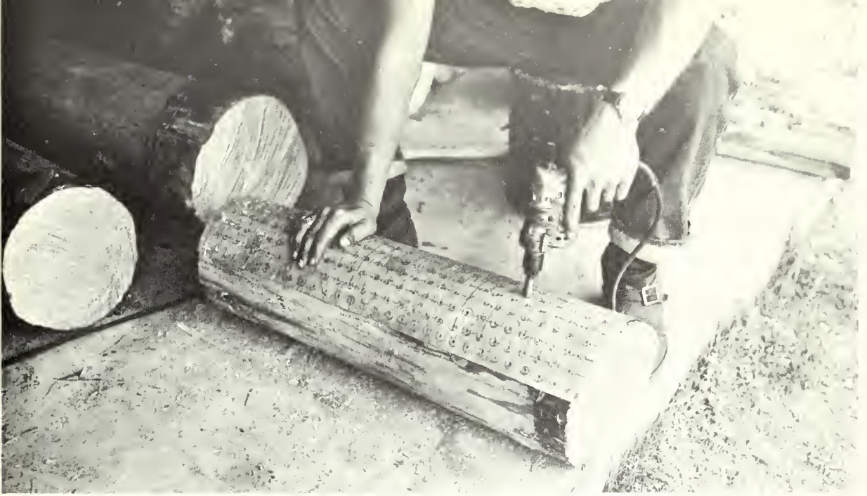
Figure 5.--Holes were bored on 1-inch centers to a depth of \frac{3}{4} inch with a \frac{1}{8} -inch drill. Even though boring proved the best of four methods tested, it would probably be more costly to bore than to incise scar-faces of full length poles on a production basis.
