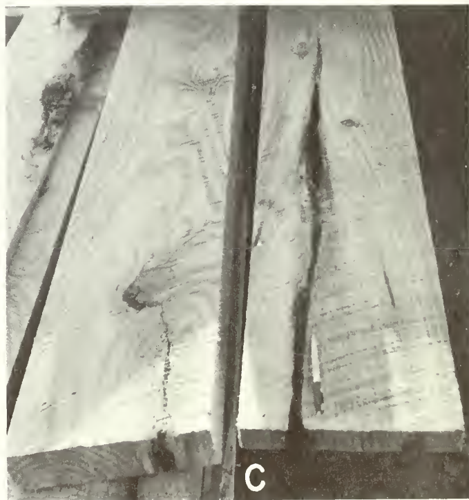
Figure 14. --Fork when left in the log, especially with included bark as in B , results in lower grade lumber. A , a fork as seen in the tree. B , fork with included bark. C , lumber from a fork as in B .
