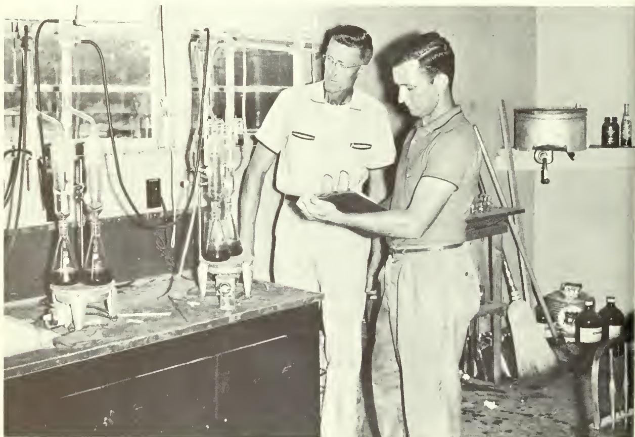
Figure 7. --Retention analysis of the cores from the test bolts was made at The Langdale Company's analytical laboratory. Toluene was used for extraction. The cores were placed in the extraction apparatus, heat was applied and the toluene was refluxed at a rate of 1 drop per second for 1 hour 45 minutes. Cores were then removed from the apparatus and placed in an oven to dry for 1 hour at 125° C. They were then removed to a desiccator for 15 minutes. Four drops of Nekl NS (sulfonated aliphatic polyester) were used to remove the water from the condensing tube. Five Interjoint Reflux condensers were used in the distillation process.
