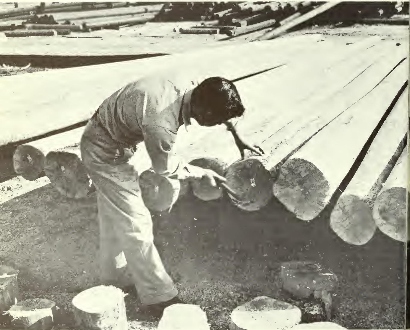
Figure 8. --Sample poles were peeled, rossed, and stacked to dry on The Langdale Company's pole seasoning yard. The average moisture content for Lot I poles just before treating was 20.1 percent, for Lot II poles 19.6 percent, for Lot III poles 30.7 percent, and for Lot IV poles 21.0 percent. Moisture content determinations were made with a resistance-type moisture meter on the fresh cut ends of the poles just after they were trimmed. Four determinations were made for each pole, two at the butt and two at the top, one from the heartwood area and one from the sapwood area. In a previous study, moisture content measurements made with a resistance-type meter were compared with those from the same poles made by oven drying a pie-shaped disc, and for most readings below 30 percent the difference did not exceed 3 percent.
