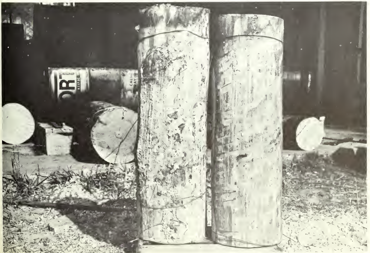
Figure 6.--A heavy deposit of gum similar to that appearing on the test bolt at left was almost completely removed by soaking either in hot caustic or hot turpentine. The bolt on the right was treated with a 3-percent solution of sodium hydroxide at 175^{\circ} F. for 4 hours. Group D bolts were kept in hot gum turpentine ( 165^{\circ} F.) for 6 hours.
