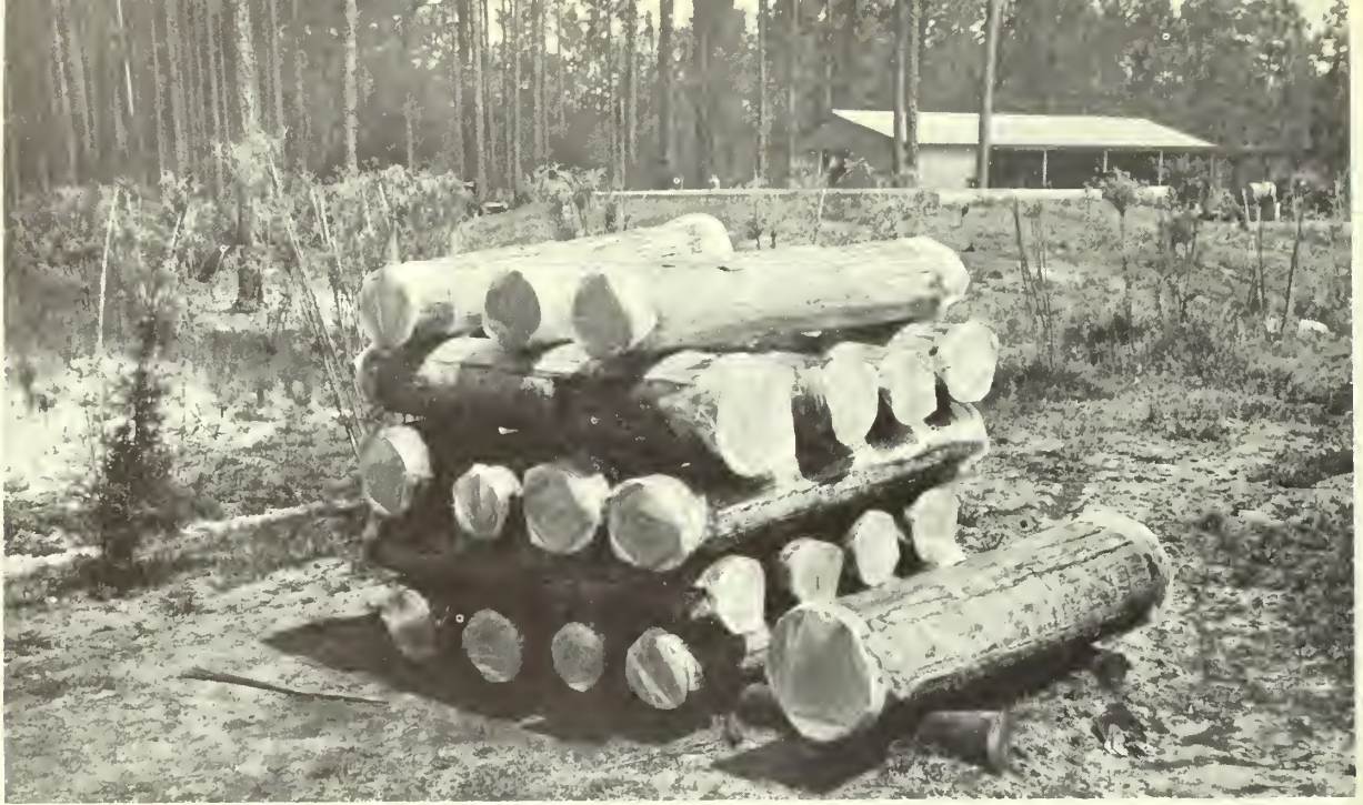
Figure 3. --The moisture content of these bolts, which were air-dried, ranged from 20.0 to 38.6 percent and averaged 28.1 percent when pretreated. The ends of the bolts were coated with an aluminum-asphalt roof coating compound containing asbestos fibers, and then wrapped in a polyethylene film to prevent excessive end checking.
