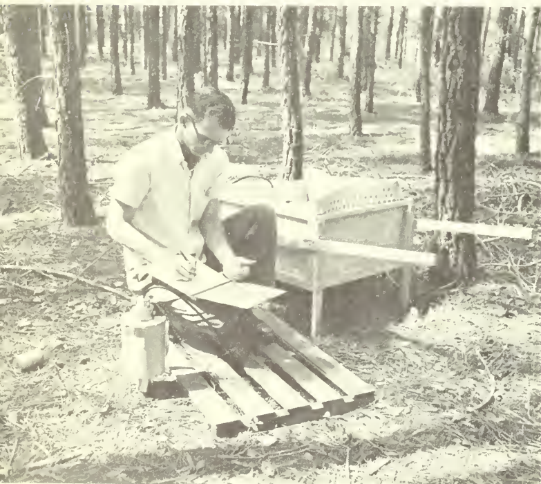
Figure 1.--Moisture content was determined with the Nuclear-Chicago Corporation P-19 Moisture Probe and Model 2800 Scaler. Spacing and relative size of the stand is shown in background.
