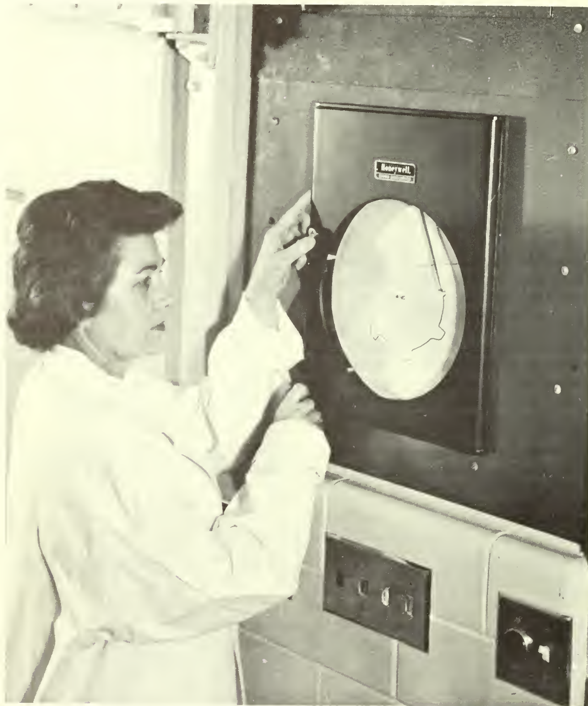
Figure 1. --Temperature and light were controlled automatically. Thermograph shows temperature in the alternating germination room.
