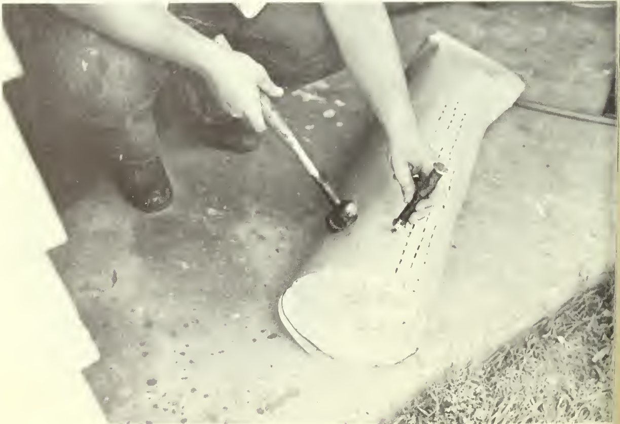
Figure 4. --This homemade hand incisor had a "chisel-point" tooth \frac{1}{8} inch wide, \frac{1}{2} inch long, and \frac{3}{4} inch deep. The test bolts were incised on 1-inch centers. Hand incising is slow and laborious. It is reported that a machine method of incising only the scar-face has been devised for commercial operations.
