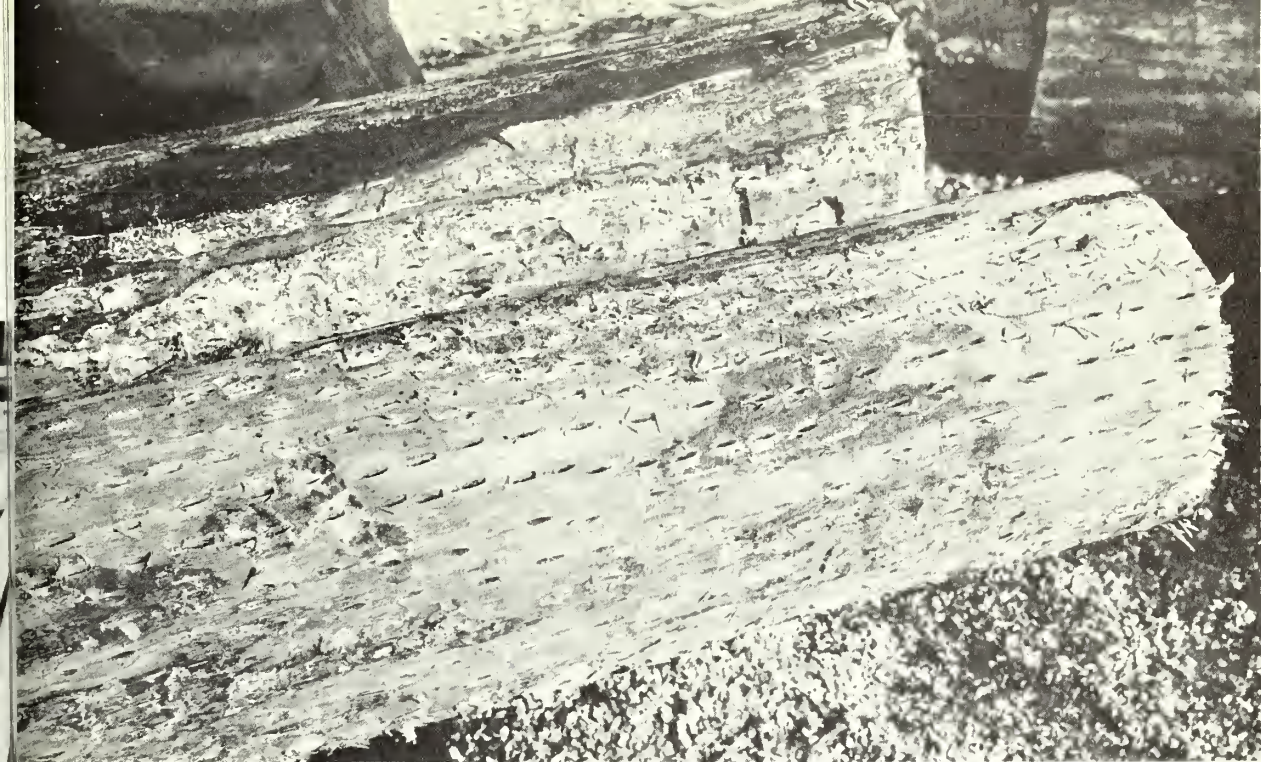
Figure 9. --The scar-faces of all poles in Lot I and Lot III were incised. Incisions were made in parallel rows approximately 1 inch apart and running the length of the face. The vertical distance between incisions was about 1/2 inch. Depth of incision was 3/4 inch, the length of the chisel-point tooth.
