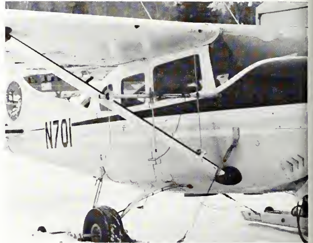
Figure 13.—Directional yagi antennas fastened to the wing struts of the aircraft were necessary to “home in” on the wolves. (Photo courtesy of U.S. Bureau of Sport Fisheries and Wildlife.)
