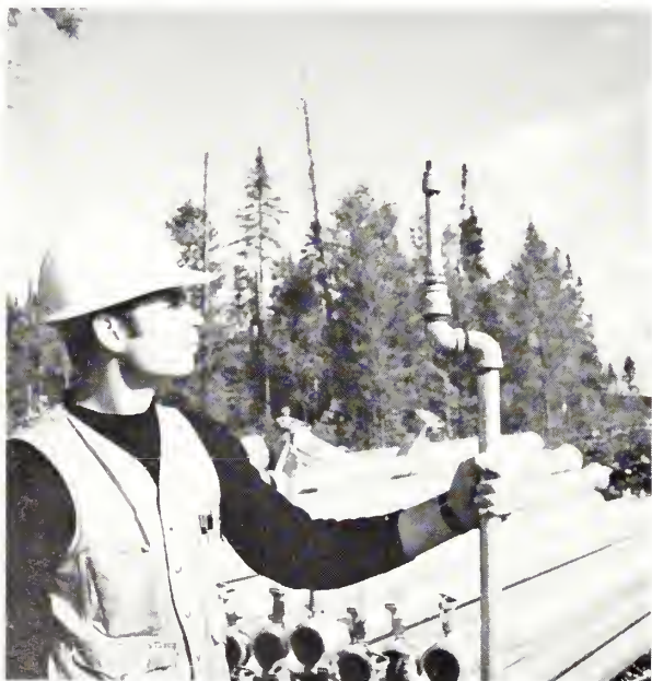
Figure 7.—Nozzle assembly consists of two iron pipe elbows, two bell reducers, two bushing reducers, one 8-by 1/2-inch nipple, and a brass nozzle head.
