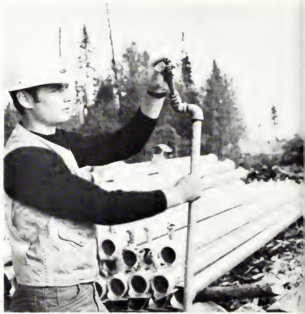
Figure 8.—The nozzle is adjustable through a 360-degree vertical arc.
