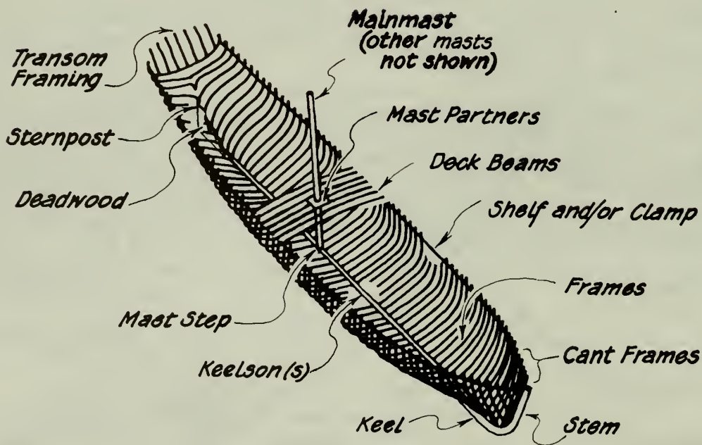
Sketch of Generic Wooden Ship Construction
