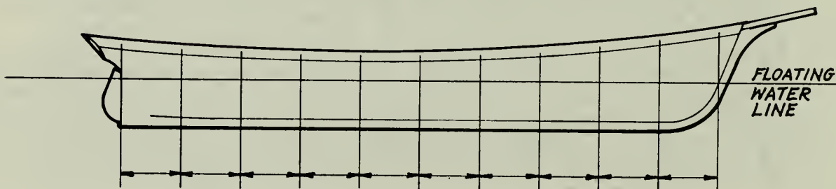
DIVIDE LENGTH OF HULL AT FLOATING WATER LINE INTO EVEN NUMBER OF EQUALLY SPACED INTERVALS (10 IS COMMON)
