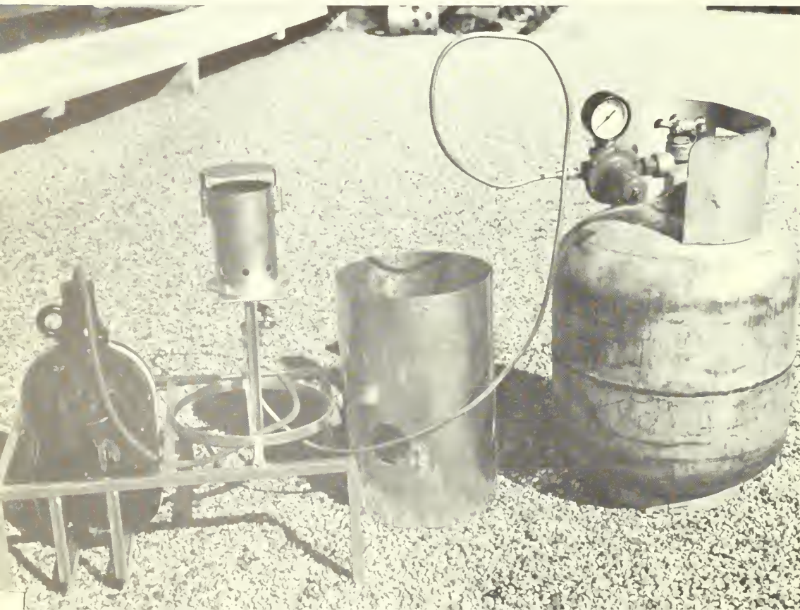
Figure 3.--Skyfire generator showing from left to right the solution reservoir, framework, flame holder, windshield, and propane supply tank.
