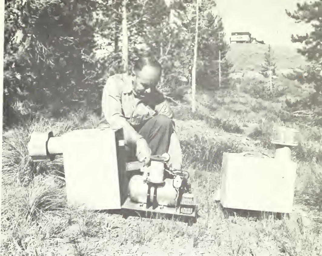
Figure 2.--String-burning silver iodide generator.
