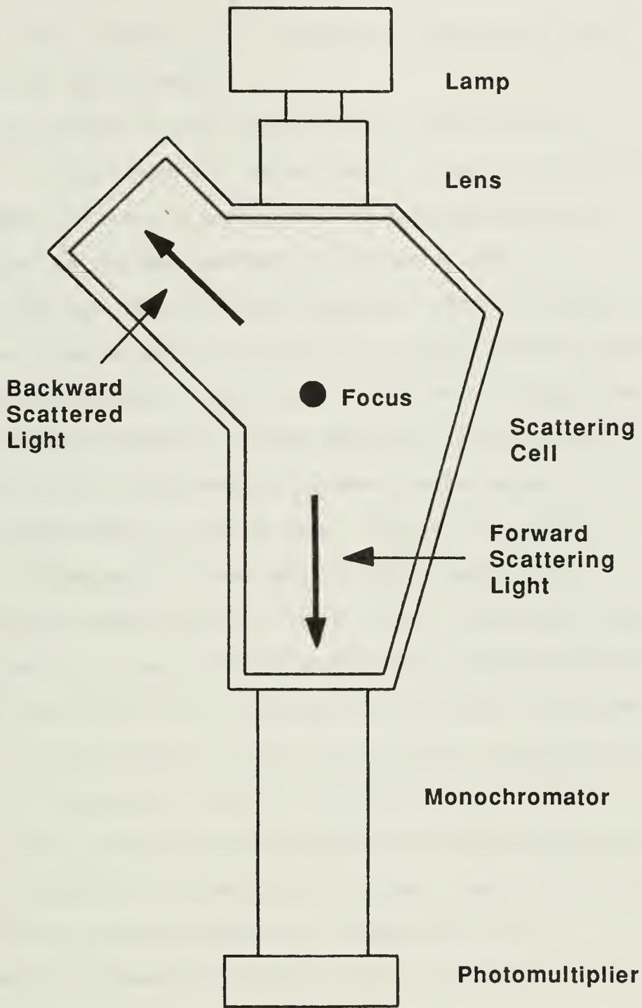
Figure 15. Diagrammatic representation of the scatter cell used in the lake color experiments.
