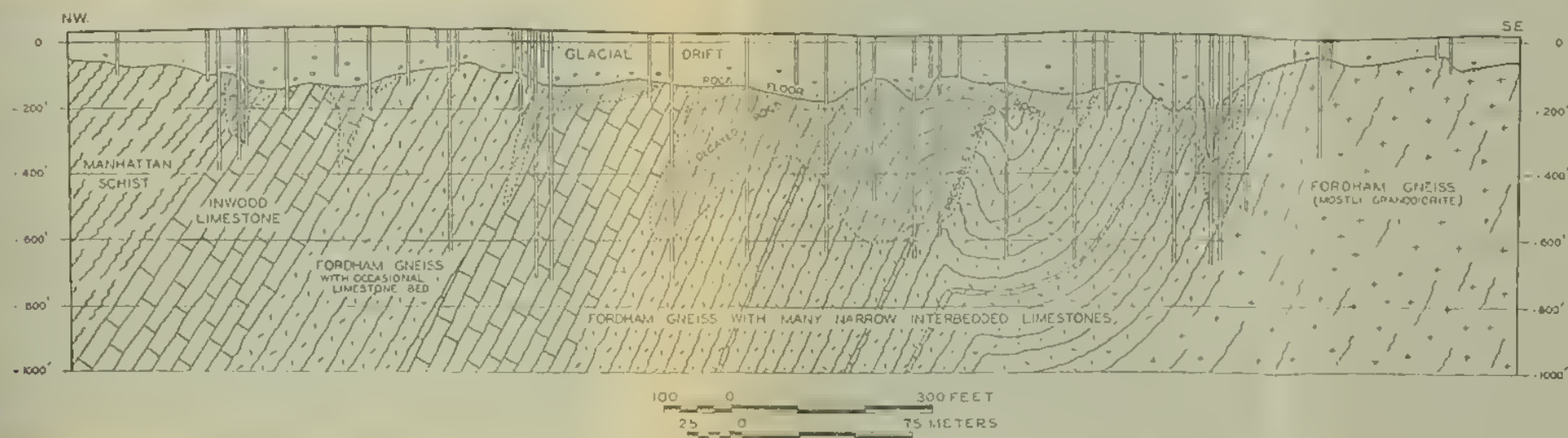
GEOLOGIC SECTION OF LOWER EAST SIDE BASED ON EXPLORATORY BORINGS FOR THE CATSKILL AQUEDUCT
