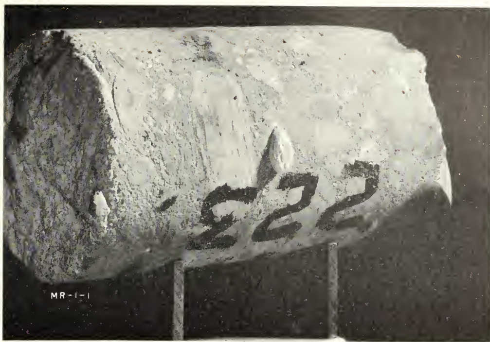
NOT BUBBLE GUM —A concrete core showing sodic-silica jell oozing out of expanding concrete—the result of reaction between alkali in cement and reactive aggregates. At right, characteristic random pattern cracking caused by expanding concrete.
