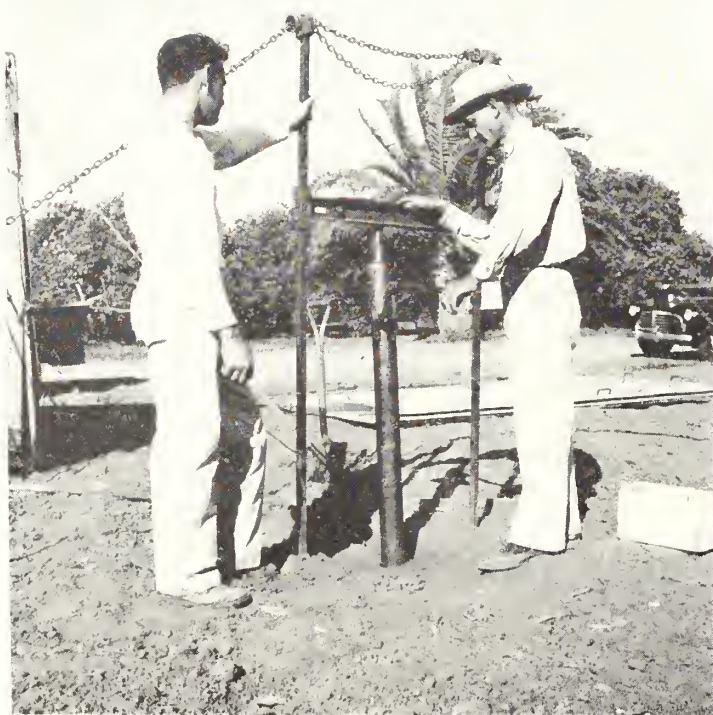
At left: "Undisturbed" soil sampling device completely assembled. The tube, with an inner tube made of 6-inch segments, is being forced into the ground with a hydraulic jack. The supports are soil augers held down by chains. Below: Measuring run-off sample during infiltration test. Sample is being poured into graduated measuring cylinders. Man at right is pressure valve attendant.
