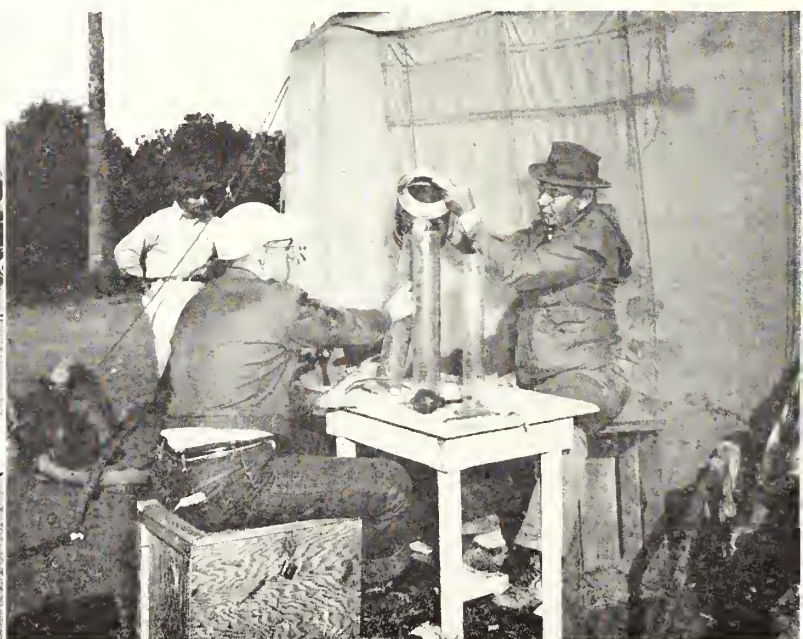
At left: "Undisturbed" soil sampling device completely assembled. The tube, with an inner tube made of 6-inch segments, is being forced into the ground with a hydraulic jack. The supports are soil augers held down by chains. Below: Measuring run-off sample during infiltration test. Sample is being poured into graduated measuring cylinders. Man at right is pressure valve attendant.
