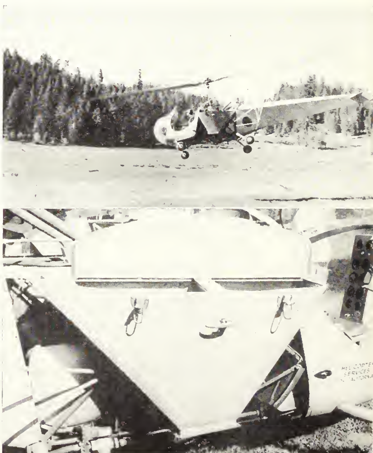
At left: Slides showing number of 2, 4-D droplets sprayed from plane at different dosage rates per acre. Below: Helicopter lands for refill on mountain meadow, inaccessible to ordinary plane. Bottom photo: Spray hopper on side of helicopter fuselage. All photos courtesy State of California Department of Agriculture.
