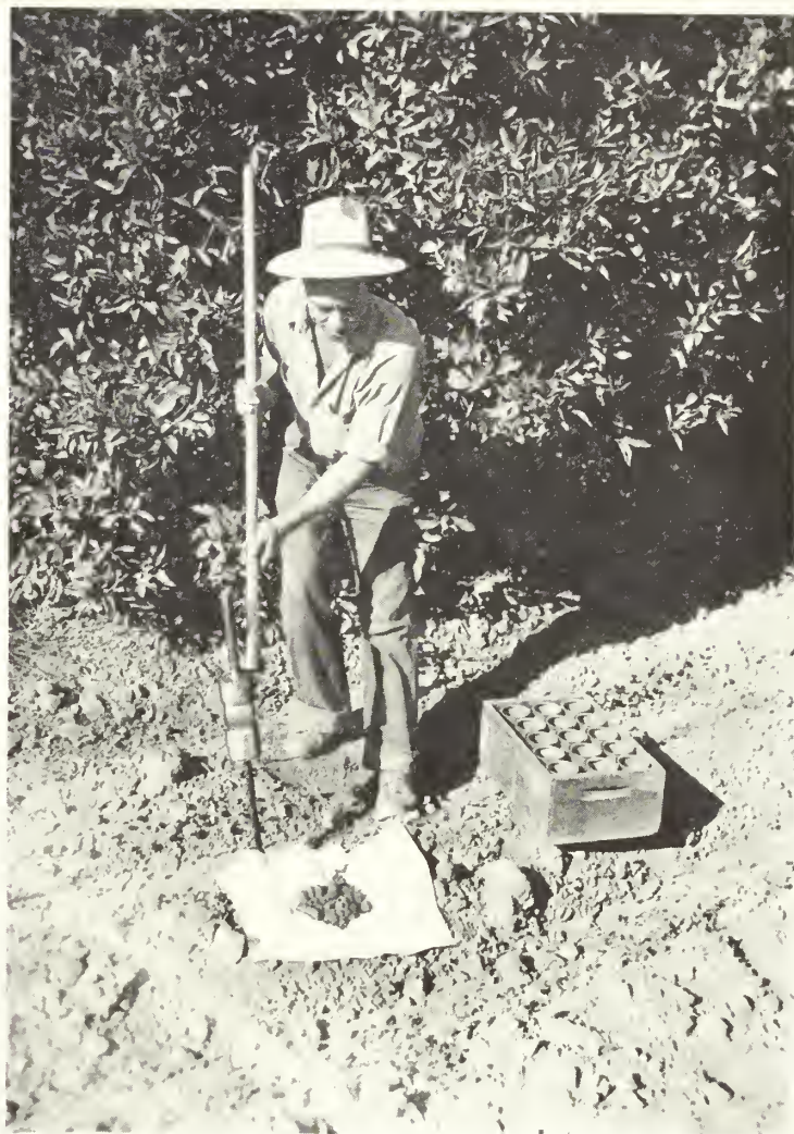
Soil samples to determine moisture content are taken from 0-12-inch zone and 12-30-inch zone in citrus groves with a third and deeper sample taken in walnut groves. Two samples are taken at each site and mixed together to yield a composite sample. Photo by A. J. Burrows, Region II.
