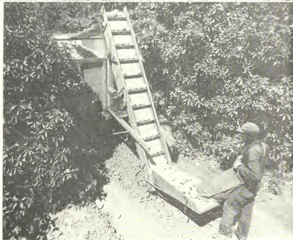
Above, mechanical loader, brain-child of Harry Ellis, Yuma Fruit Growers Association, which saves precious time in getting fruit on its way. Right, petite packer Dorothy Tschilar of Phoenix, one of the fastest in the business. Photos by Harry W. Myers, Region III.
