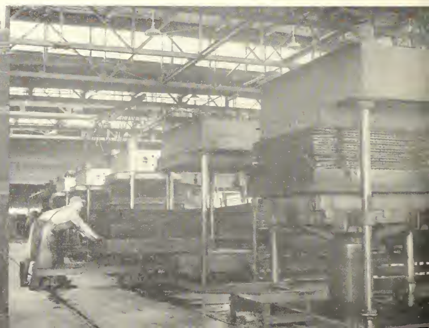
Closeup of six huge presses which squeeze the grape juice from the mash.
