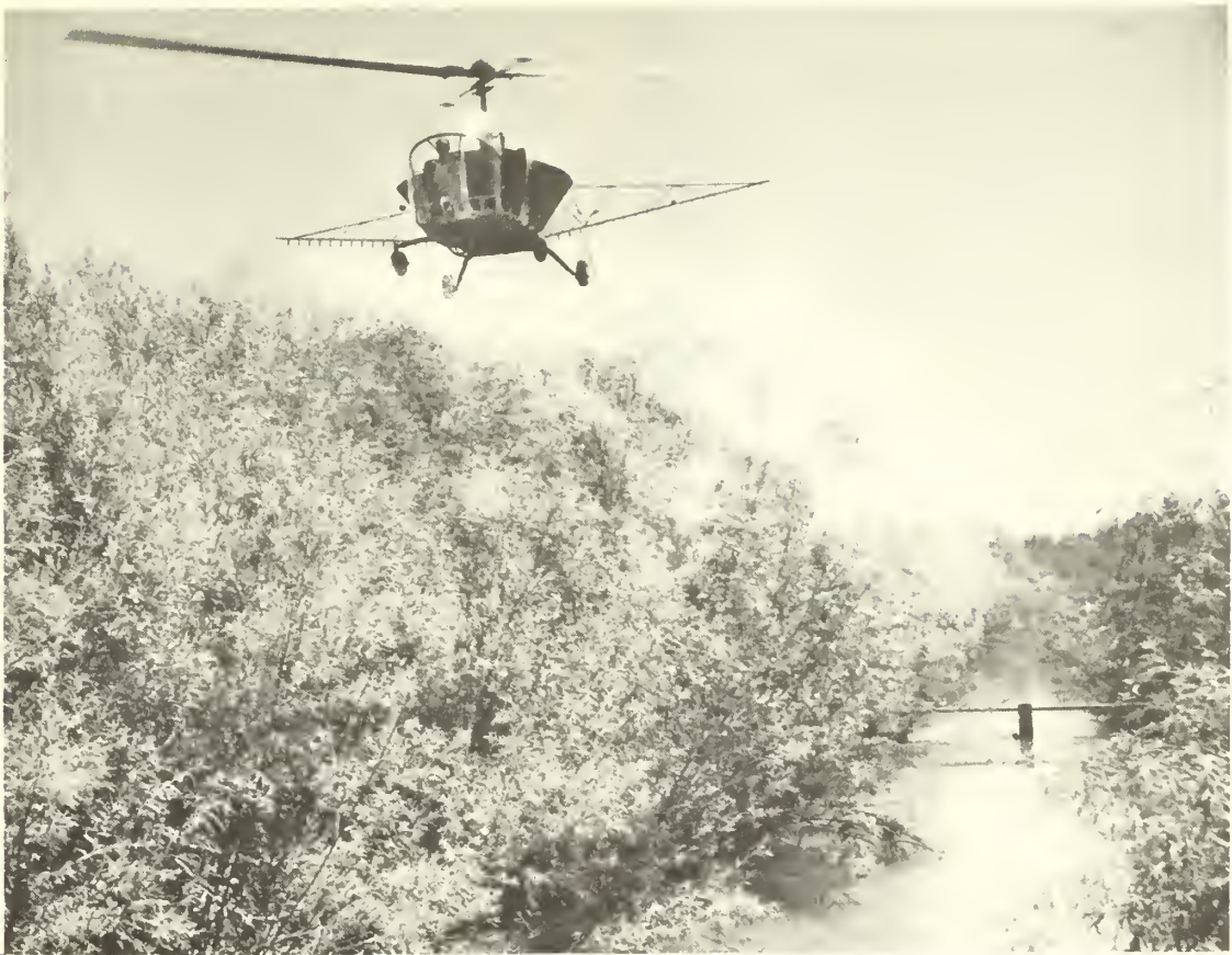
A helicopter is ideal for applying low-volume chemical sprays on phreatophyte growth along irrigation and drain canals, especially where there are no ditchbank roads (Bureau of Reclamation Region 6).
