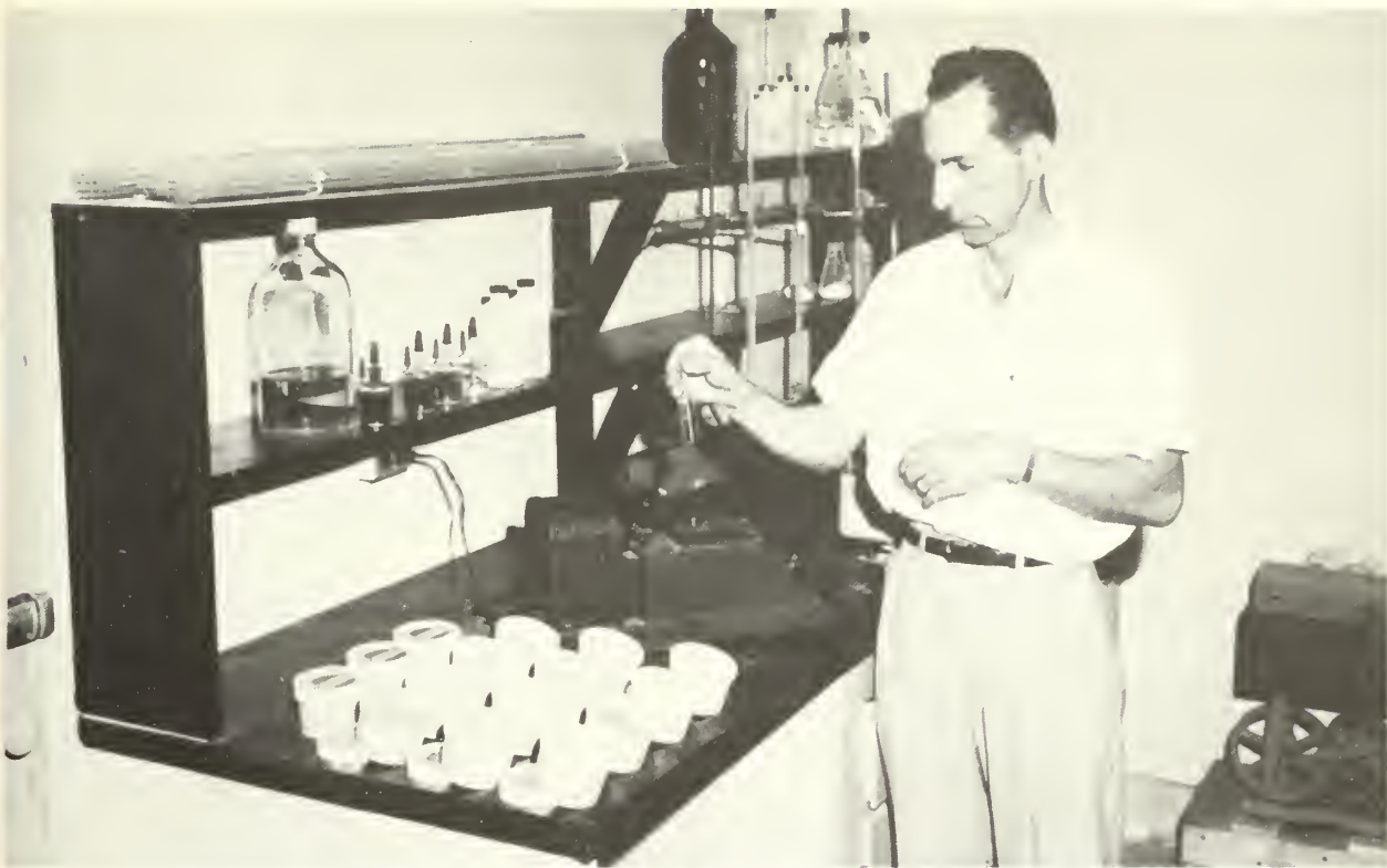
V. H. Gledhill, New Mexico A & M College, is using a photoelectric colorimeter to determine phosphorus in soils.
