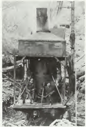
Massive steam-powered skidders pulled logs in off the hills to a central pile. Then the loaders took over and put the logs on trains, which carried them to the mills.
