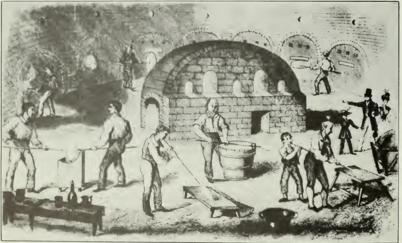
Figure 122. Crown Glass Manufacture (a, rolling the "eye"; b, flattening the globe of glass; c, attaching a puntty to the flattened end of the globe; d, spinning the globe into a flat disk of glass (Diderot 1959:plates 241, 242, 243, 245)).
