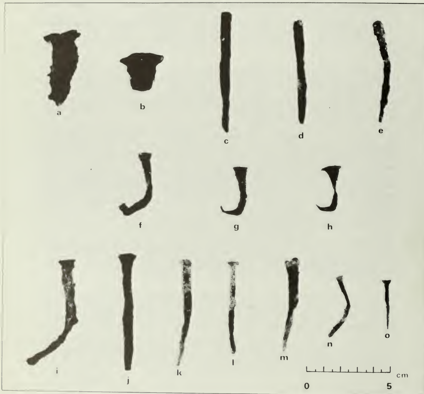
Figure 118. Nails and Spikes (a and b, handwrought spike fragments; c, d, and e, headless machine-cut nails; f, g, and h, machine-cut clinch nails; i to o, common machine-cut nails).
