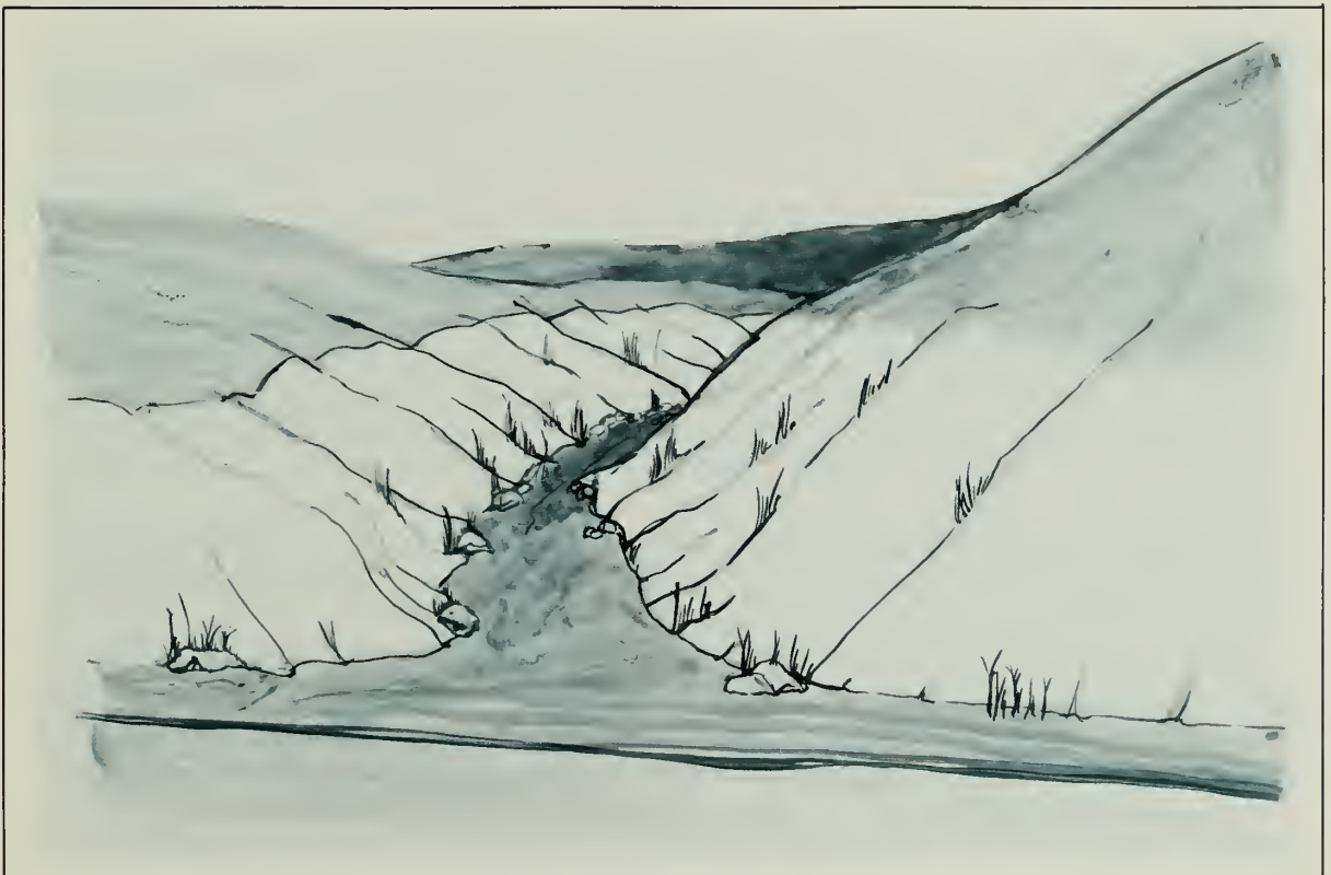
Lay-back draw; cut slope flattened to match slope of draw
