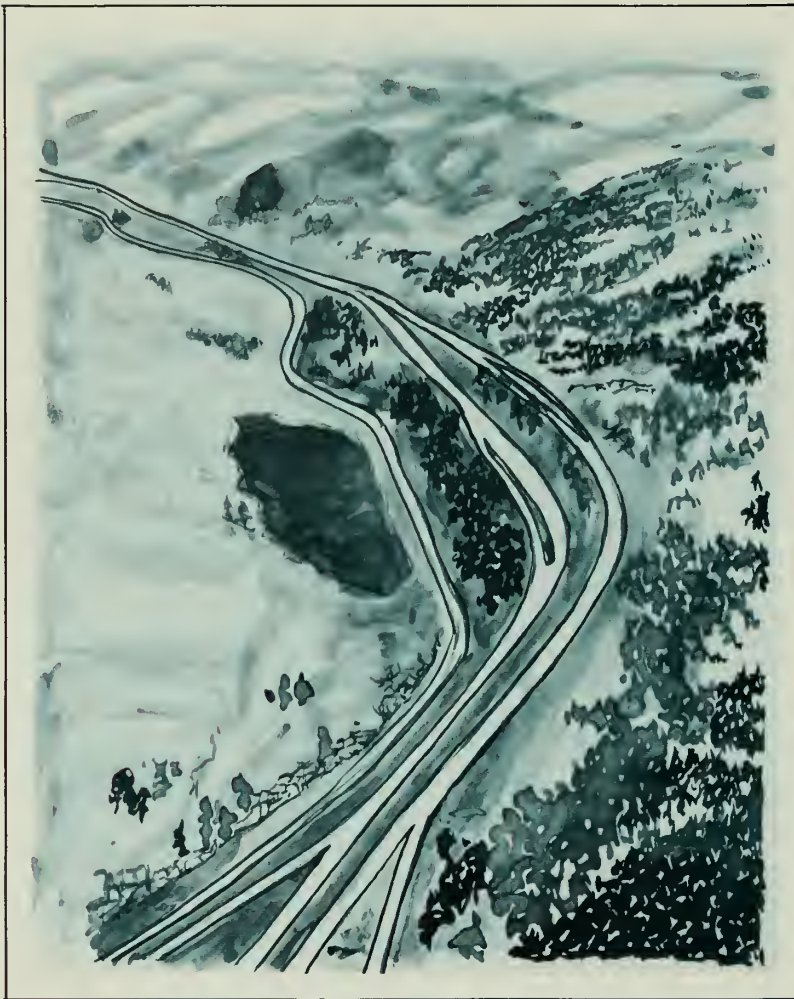
Varying median widths – 4-lane facility with adjacent service road
