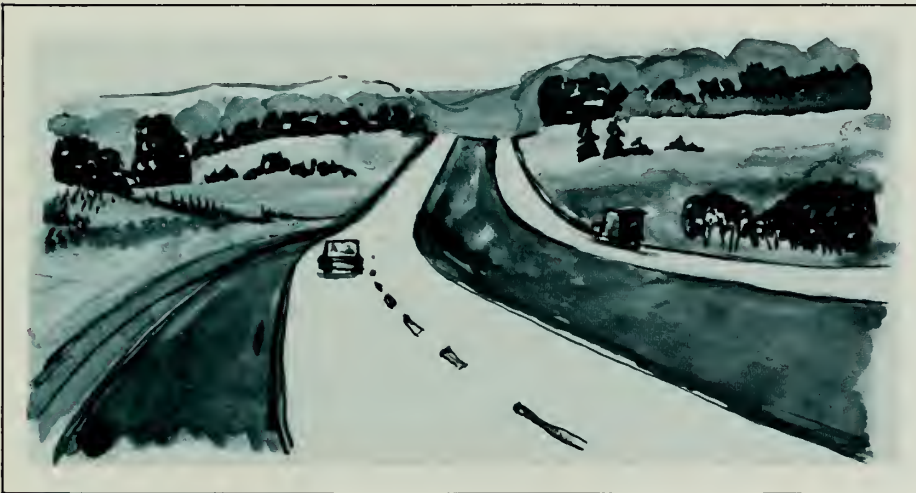
Coordination of horizontal and vertical alignments
