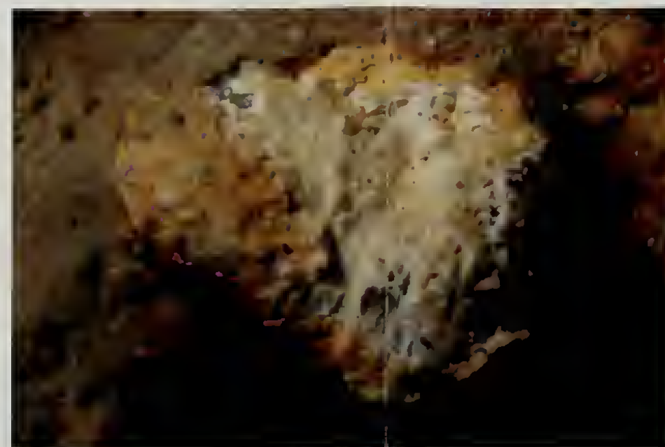
North Dependency, micrograph of finishes on pebble-dash stucco
