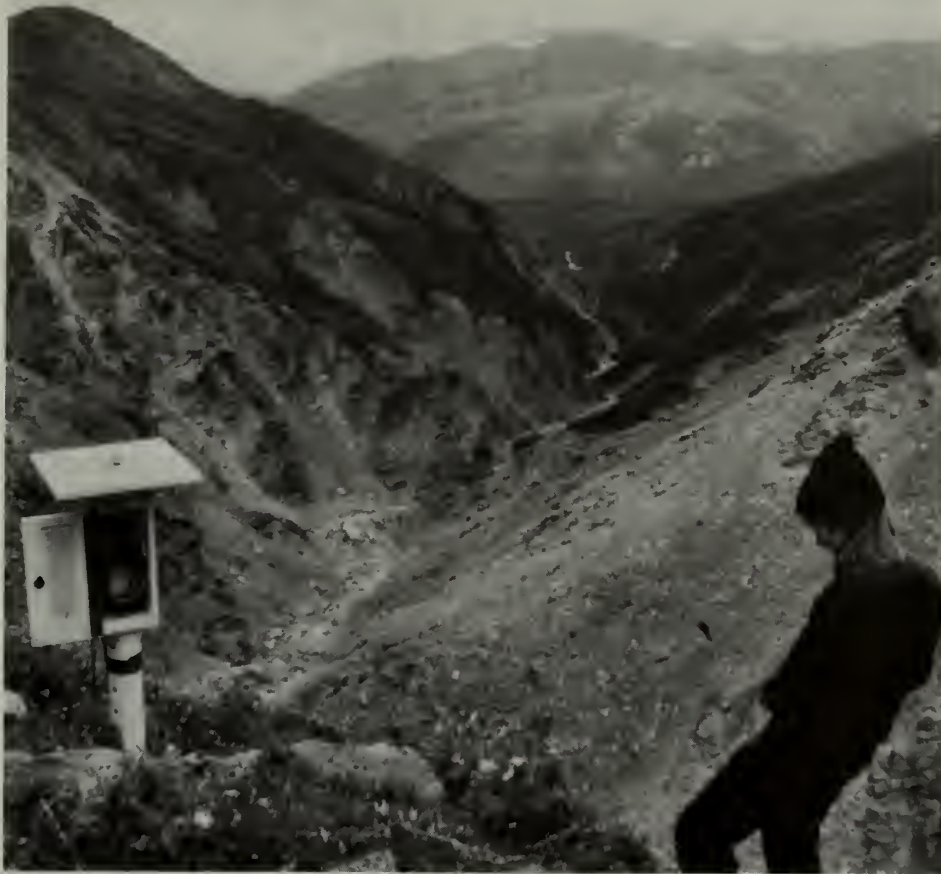
Figure 2. Remote automated monitoring station to assess effect of temperature, moisture, and radiation on vegetation production, decomposition, and nutrient cycling.
