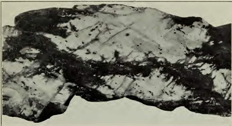
A. POLISHED SPECIMEN OF PEGMATITE SHOWING REPLACEMENT BY FERROMAGNESIAN MINERALS ALONG SHEAR ZONES
