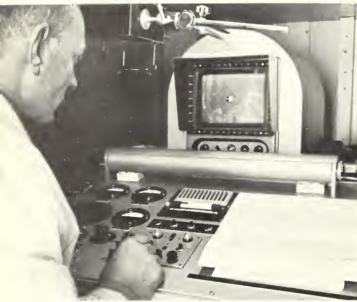
Geologist Malcolm Logan is shown viewing the screen of the TV borehole telescope which is in the ground approximately 70 feet.
