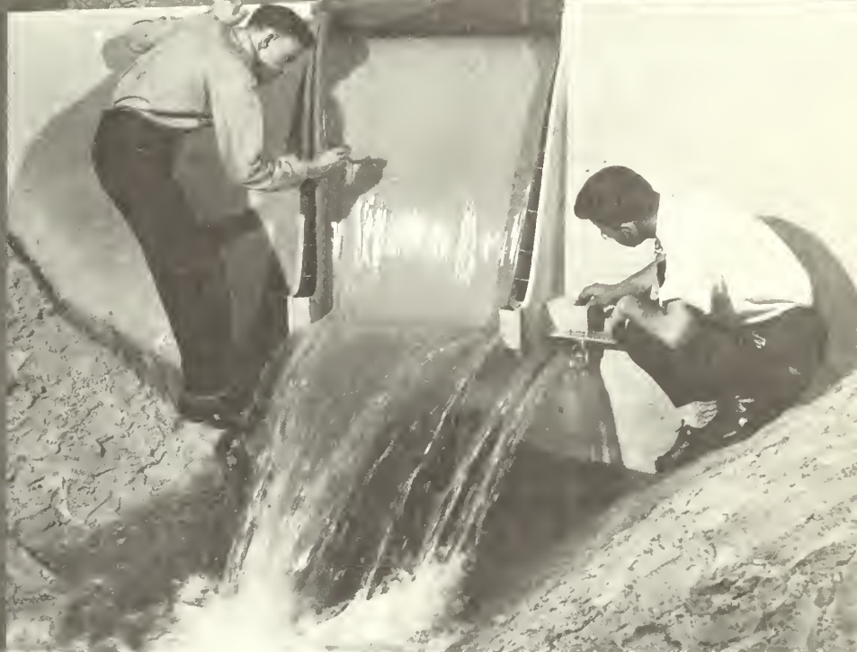
The "ski-jump" or flip bucket model of the base of the overflow spillway at Anchor Dam, Wyoming.
