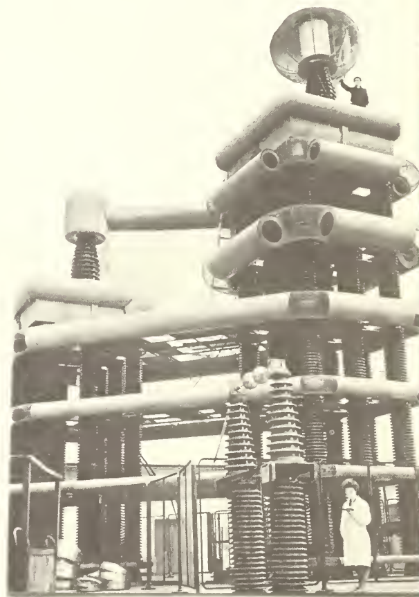
Cascade of transformers for testing at 2,250 kv. at Moscow.
