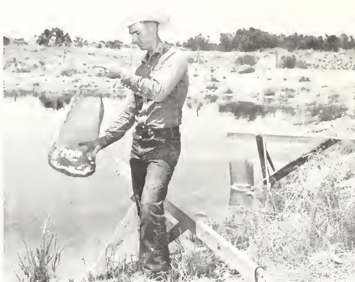
Two copper mesh bags are used in this experiment to properly confine the chunks of solid emulsion evaporant.
