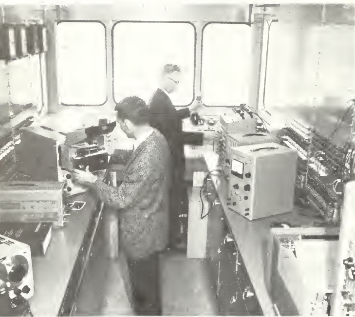
Inside equipment includes console for control of power apparatus; also public address system, radio, telephone and auxiliary power set.
