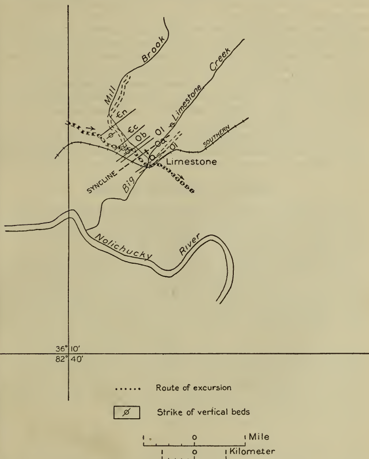
FIGURE 9.—Map and section along Mill Brook 1 mile (1.6 kilometers) northwest of Limestone, Tennessee. Shows a fully exposed section from Nolichucky shale to Athens shale. Oa, Athens shale; Ol, Lenoir limestone; Ob, Beekmantown limestone; Ec, Conococheague limestone; En, Nolichucky shale.
