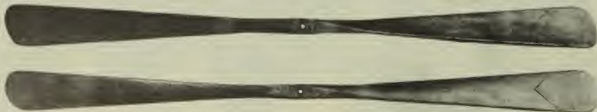
Propeller estimates, made by the Wrights 8 months before the flights of December 1903. Their formulas resulted in the highly efficient propellers which were used in the first Wright Flyer. These were 8½ feet from one canvas-covered tip to the other. Top view shows the front, bottom view, the rear.
