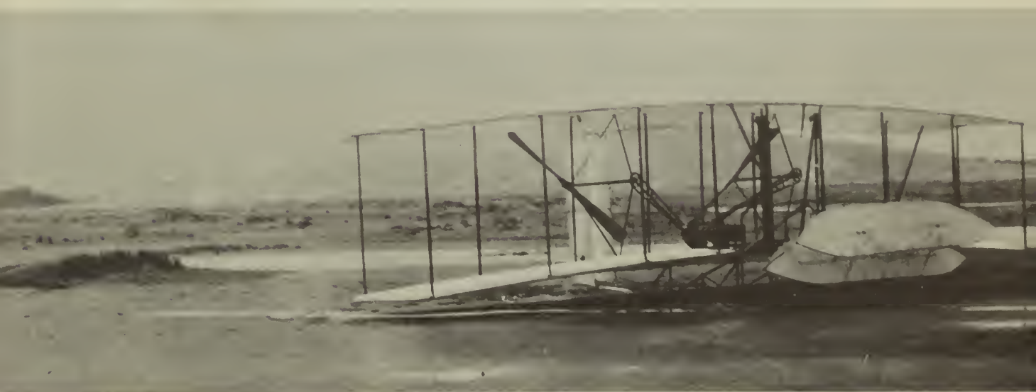
Close-up of 1903 machine at end of last flight, rudder frame broken in landing. Courtesy, Smithsonian Institution.
