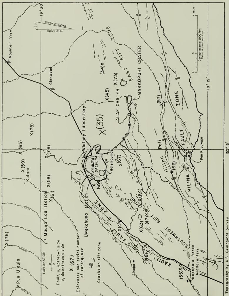
FIGURE 39.—Map of Kilauea caldera and vicinity, showing the epicenters of the large earthquake of April 22 and its aftershocks in relation to fault zones and the rift zones of Kilauea volcano. The position of the epicenter of the large earthquake (number 35) was estimated on noninstrumental grounds and its location is only approximate.
